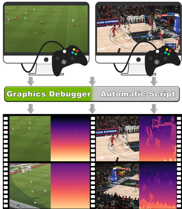
Figure 1. SoccerNet-Depth . We introduce a novel scalable dataset for Monocular Depth Estimation in sports videos. Our synthetic dataset is generated from video games, simulating football and basketball games. We leverage graphics debuggers and automatic scripts to extract video sequences along with their depth maps.
