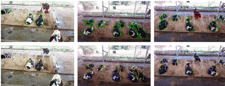
Figure 4- 1: Example annotations for cow instances (top) and flank objects (bottom). Polygons in red and green represent standing and lying cow instances, respectively. Rectangles in yellow and blue represent the flank objects on the hind leg side and the opposite side, respectively.
