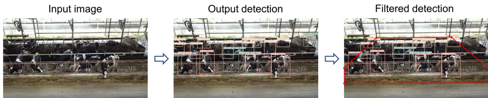
Figure 5-1: Schematic of detection filtering taking one camera for example. The predefined red polygon represents the area of interest and only the bounding boxes with their lower centres in the area are kept.
