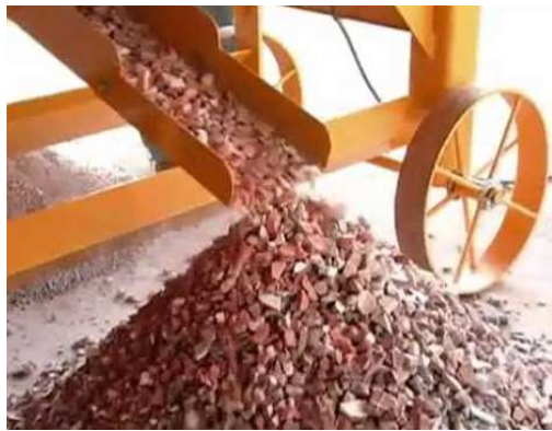
Figure 11: Recycling bricks: Crushing (Sharma, 2017)
