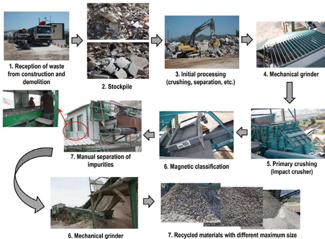
Figure 9: C&DW recycling process (source: (Medina et al., 2015))
