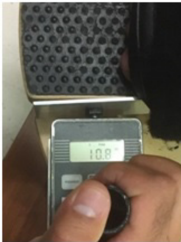
Figure 1E: Image close up of the dynamometer, placed at the medial foot side of the rotating board.
