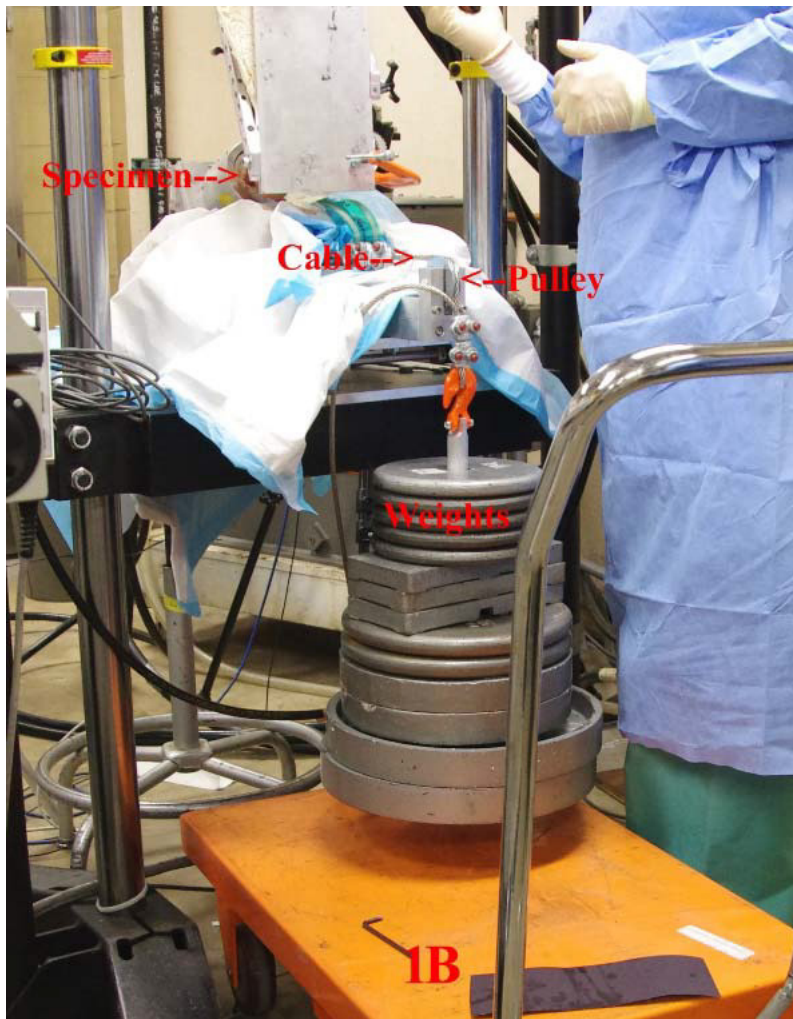
Figure 1(B). Test setup showing the cable, pulley, and weights that create the body weight axial compressive force on the foot and ankle.
