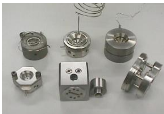
Figure 2.2: Different types of DAC among which Le Toullec, Diacell, Chervin and Akahama types.
