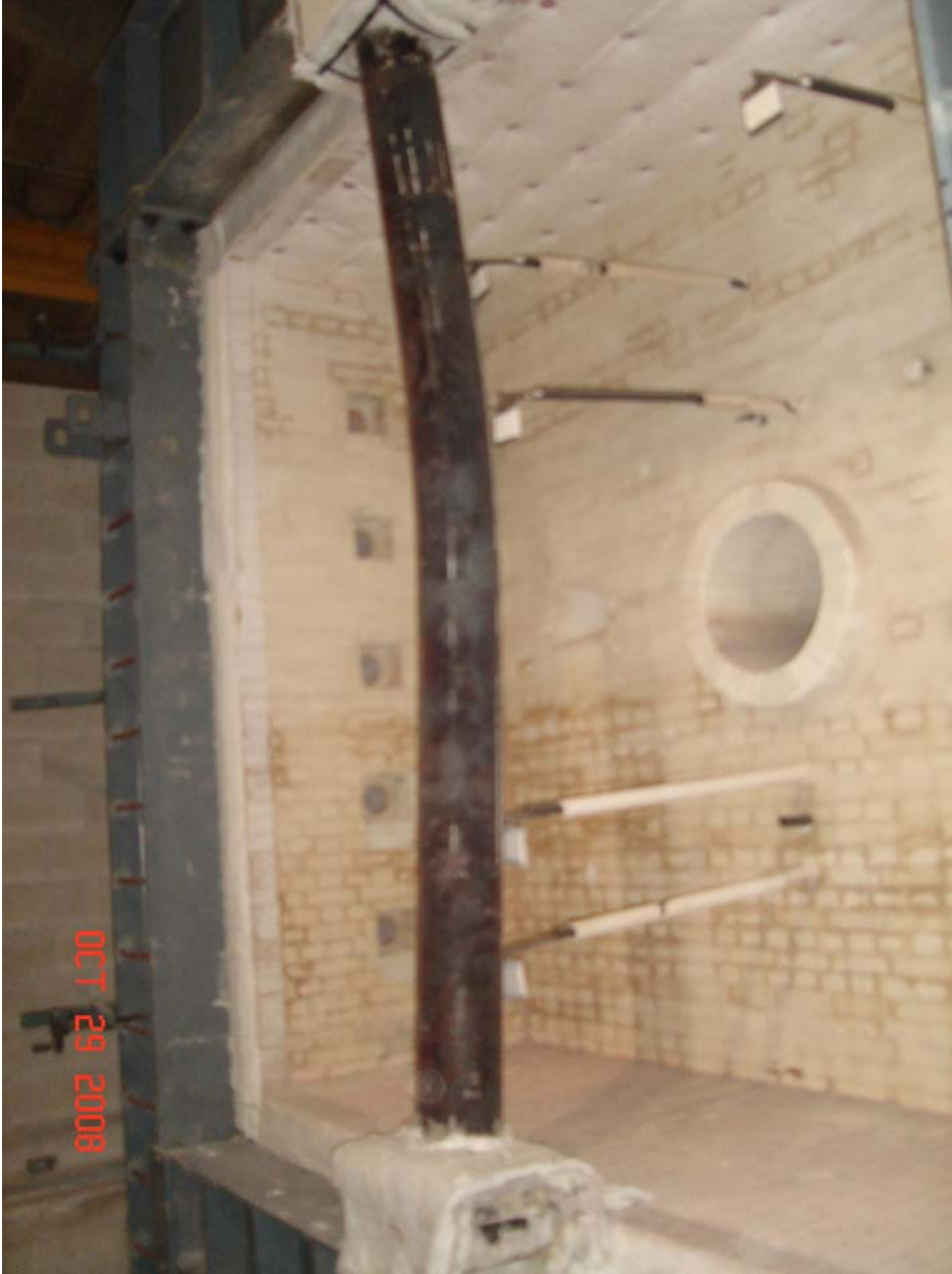
Picture A2. 2. Column FRFC 1B after the test
