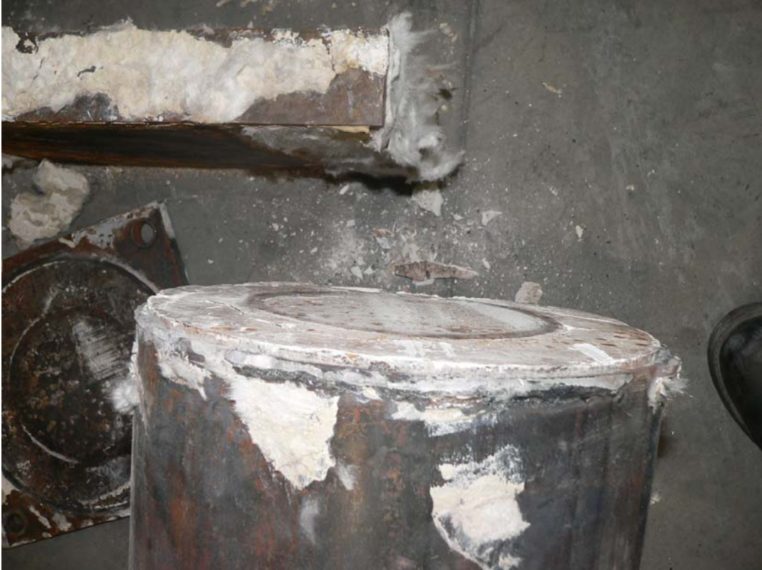
Picture A2.9. The upside of the column FRFC 5B after the test
