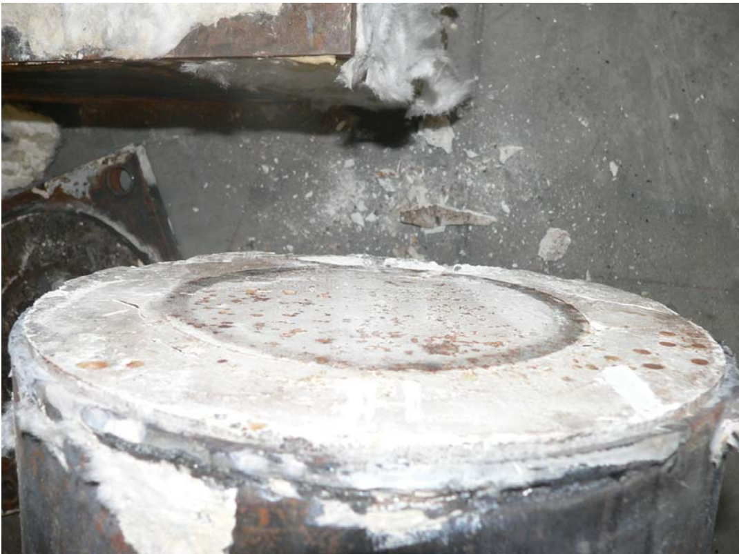
Picture A2.10. The upside of the column FRFC 5B after the test
