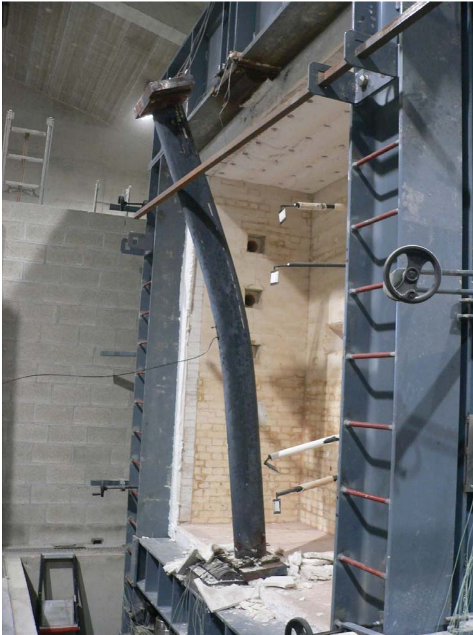
Picture A2. 1 Column FRFC 1A after the test
