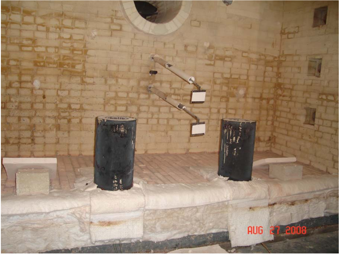
Picture A2.12. The columns FRFC 6 after the test
