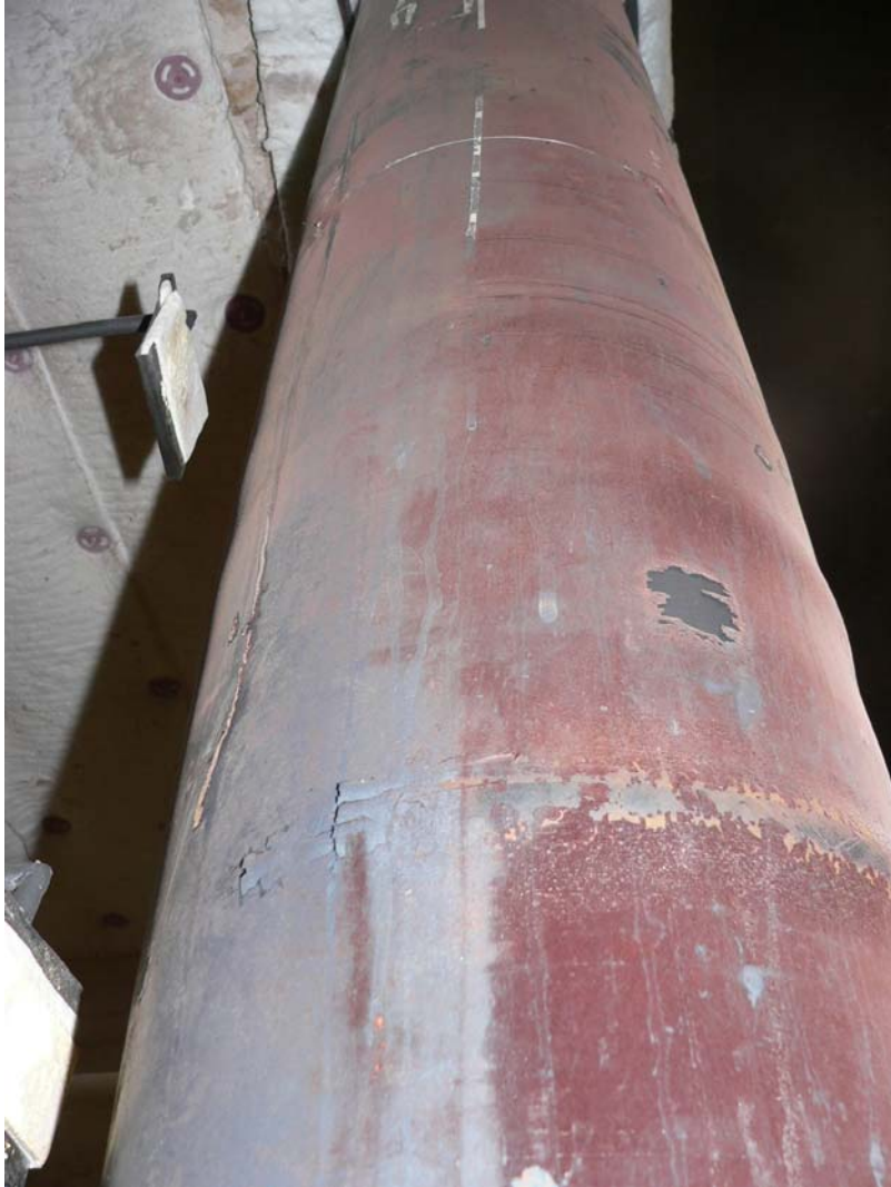
Picture A2.8. Local buckling of the test FRFC 5B
