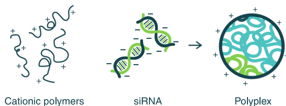
FIGURE 18.4 Formation of polyplexes by electrostatic interaction from cationic polymer and anionic siRNA.
