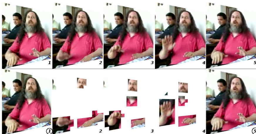
Figure 2.1: A uncompressed video flow (top) and the corresponding keyframes (1,5) and deltaframes(2-4) flow
