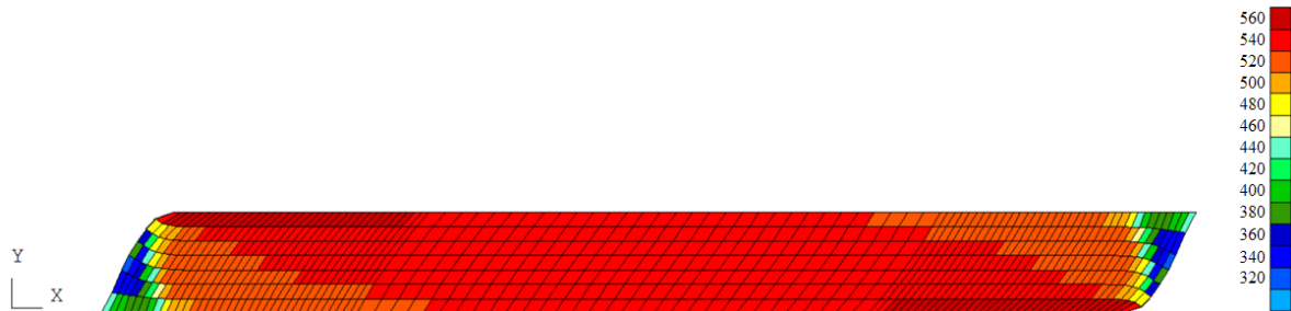
Figure 8.14: Numerical simulation of shear test with Norton (second set of parameters) - 707 FE - Distribution of \sigma_{12} (MPa) in each element after a displacement of 2.6 mm.
