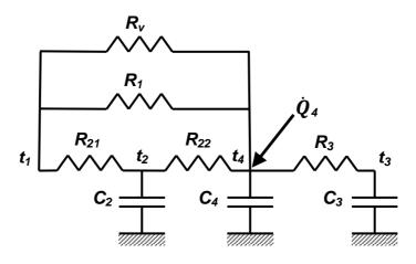
Fig. 4.5. Dynamic simplified model for a whole building zone.
