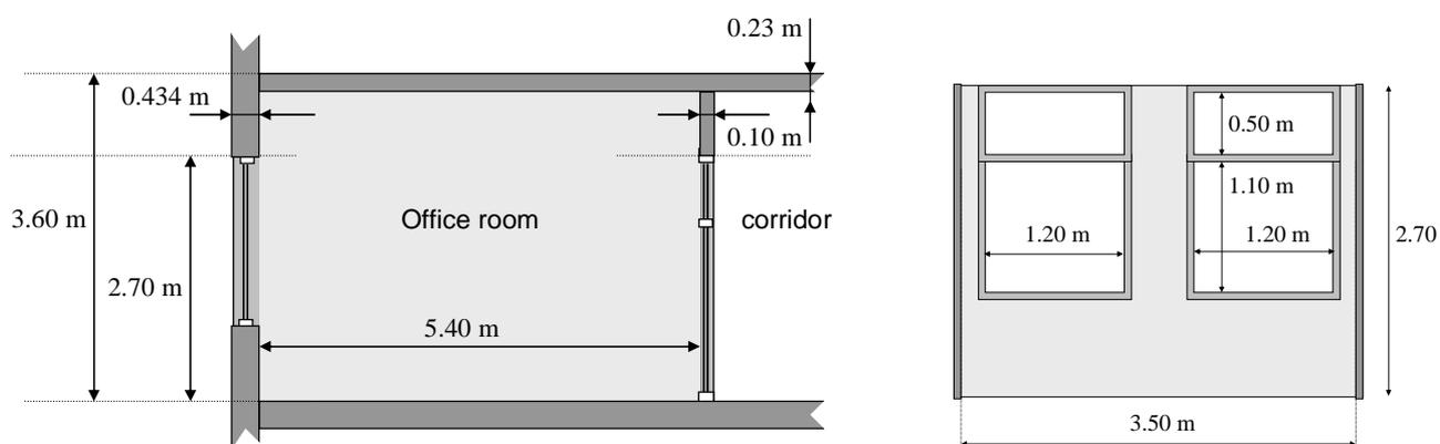
Fig. 4.4. Office room (IEA 27): section (left) and facade (right).
