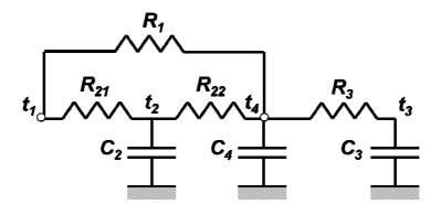
*Fig.4.2.b: One zone building model including external walls (massive and no massive) and massive internal walls.*
