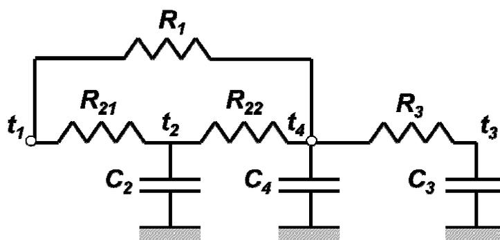
Fig.4.2.b: One zone building model including external walls (massive and no massive) and massive internal walls.
