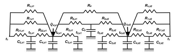
Fig. 4.6 Two zones dynamic simplified building model
