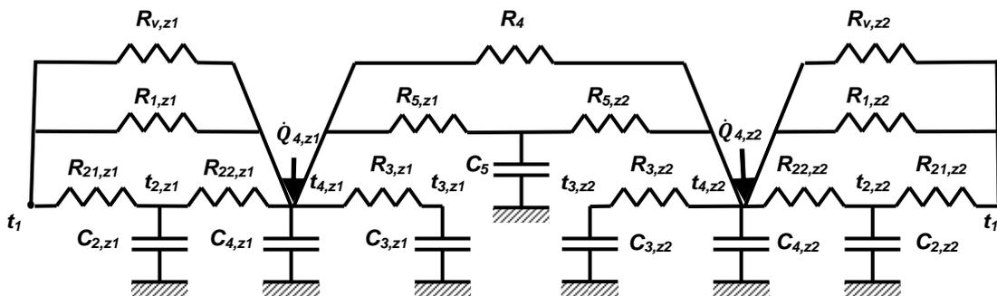
Fig. 4.6 Two zones dynamic simplified building model
