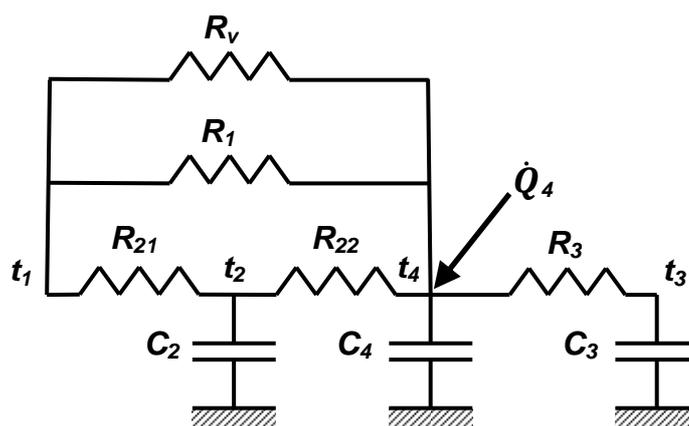
Fig. 4.5. Dynamic simplified model for a whole building zone.
