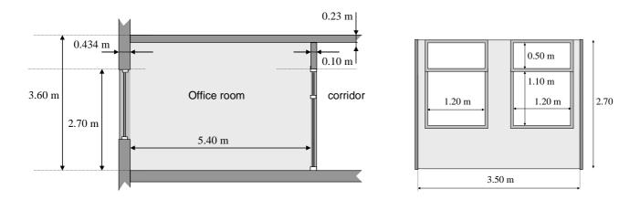
Fig. 4.4. Office room (IEA 27): section (left) and facade (right).
