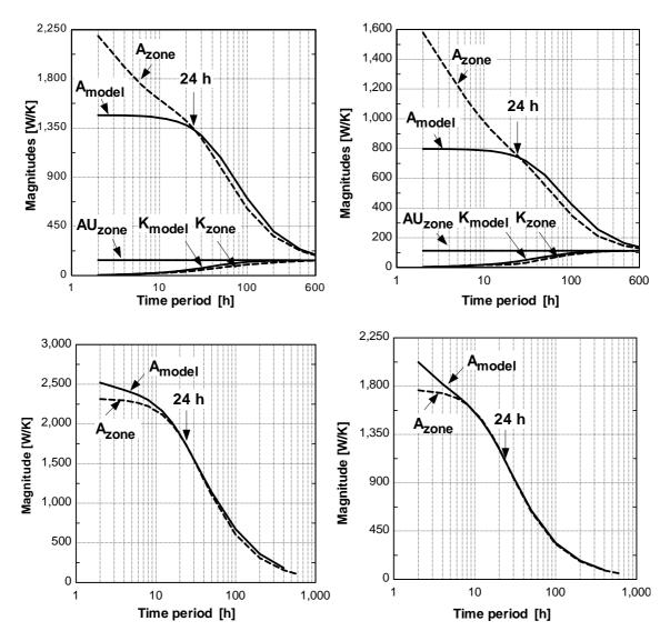
*Fig 4.3: Bode Diagrams of global isothermal transmittance and admittance (up) and of global adiabatic admittance (down) for house 1 (left) and house 2 (right) one zone models.*
