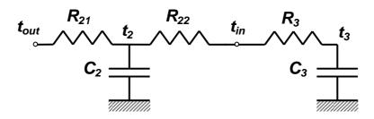
*Fig.4.2.a:* One zone building model including external walls and internal massive walls.
