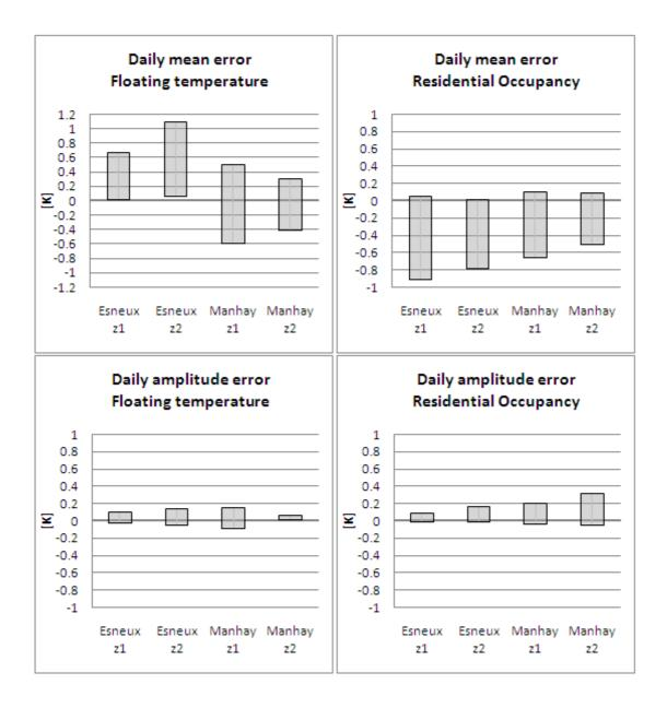
*Fig. 5.21: Confidence interval of the error on the daily mean and daily amplitude related to indoor temperature, for two zones models.*
