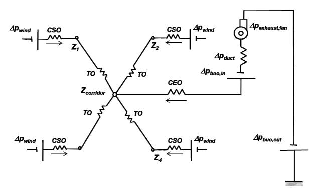
*Fig. 6.6 Type C combined ventilation model including four zones and a corridor connected to an exhaust fan.*
