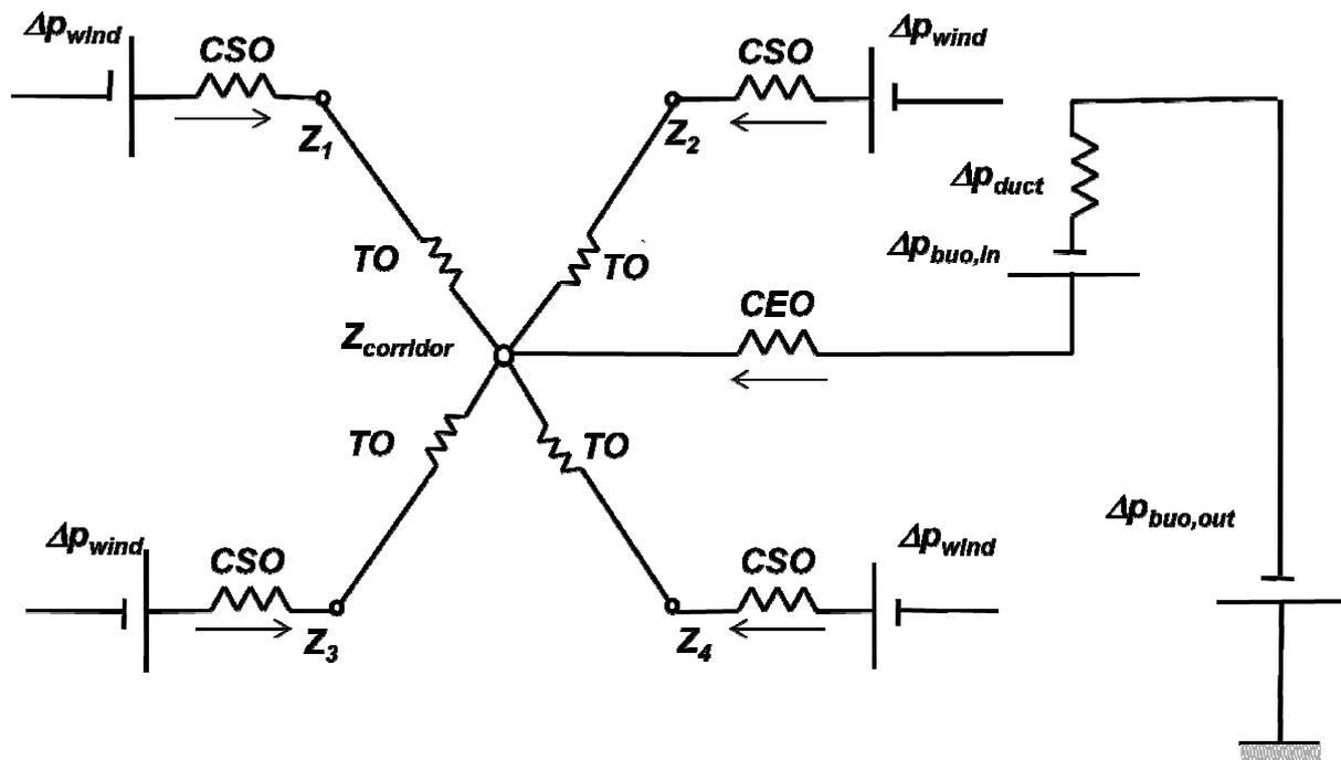
Fig. 6.5 Natural ventilation model adapted to an office building area.
