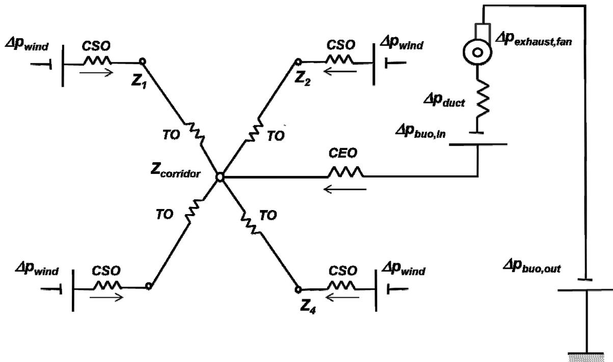
Fig. 6.6 Type C combined ventilation model including four zones and a corridor connected to an exhaust fan.
