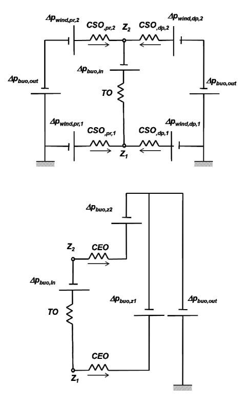
Fig. 6.1 House natural ventilation model including two zones.
