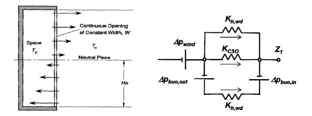
Fig. 6.2 Window stack effect (left) [38] and model of window stack effect coupled with Controlled Supply Orifices (right).
