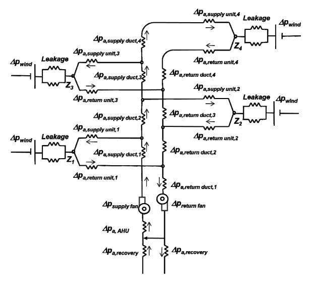
Fig. 6.7 Type D ventilation model including supply and return air ducts.
