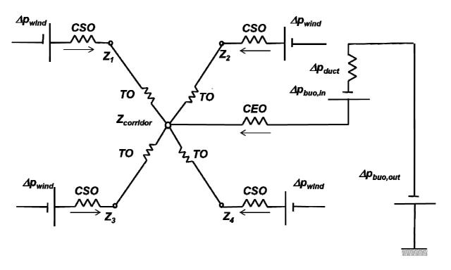
Fig. 6.5 Natural ventilation model adapted to an office building area.
