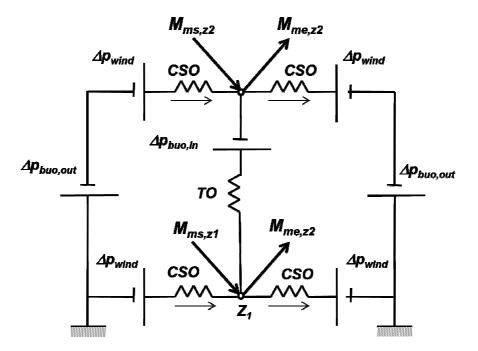
*Fig. 6.3 Model of combined natural/fan powered ventilation adapted to a house. The model must be completed with the exhaust duct branch represented on fig. 6.1 down.*
