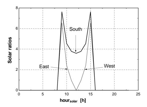
*Fig. 2.5: Solar ratios for vertical South, East and West oriented walls (full lines) on the 21<sup>st</sup> of December.*
