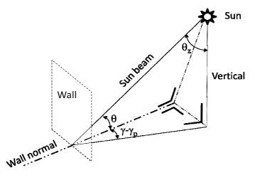
Fig. 2.1: Angles  $\theta$  and  $\theta_z$  as well as azimuth difference between sun and wall for a vertical wall  $(p=\pi/2)$ .
