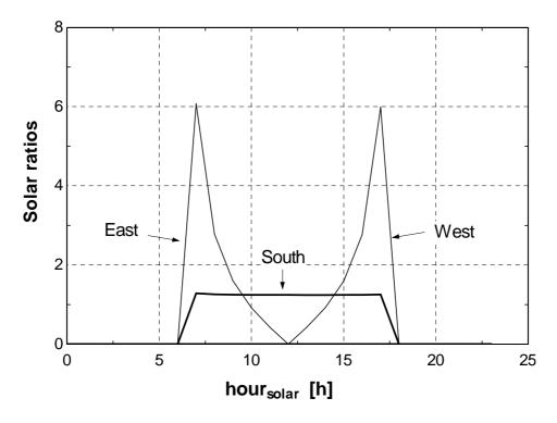
*Fig. 2.4: Solar ratios for vertical South, East and West oriented walls (full lines) on the 21<sup>st</sup> of March.*
