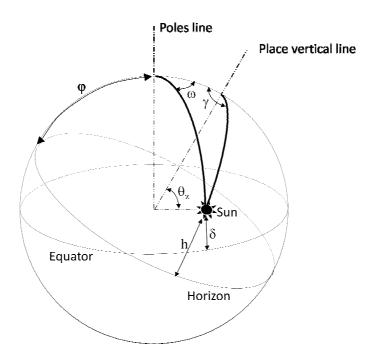
Fig. 2.2: Angle  $\theta_z$  as function of sun declination  $\delta$ , latitude  $\varphi$  and true solar time  $\omega$
