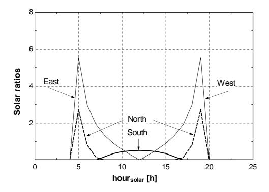
*Fig. 2.3: Solar ratios for vertical South, East and West oriented walls (full lines) and for vertical North oriented wall (dotted line) on the 21<sup>st</sup> of June.*
