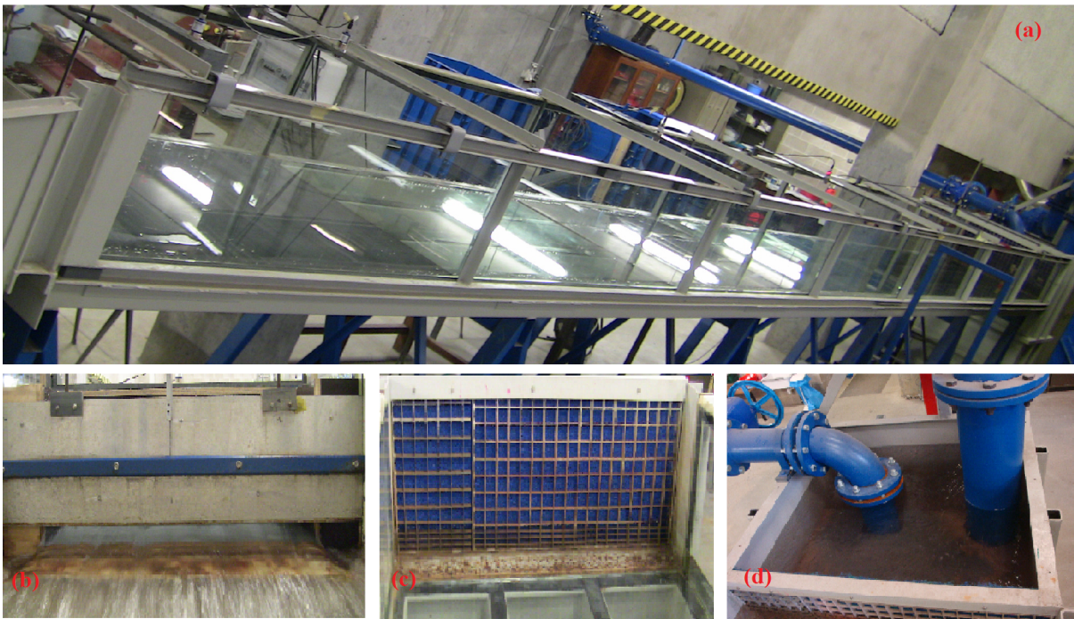
Figure 3.8: Photos of the experimental facility: (a) general view of the main flume, (b) sluice gate, (c) permeable screen, and (d) upstream stilling tank and water supply pipes
