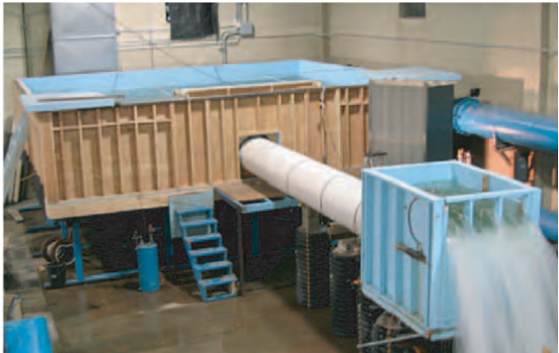
Figure 2.21: Overview of physical model with a circular conduit [76]
