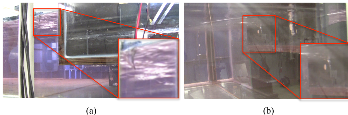
Figure 7.5: Views of vertical vortex and air entrainment in front of the conduit mouth of the physical model: (a) asymmetric geometry, (b) symmetric geometry
