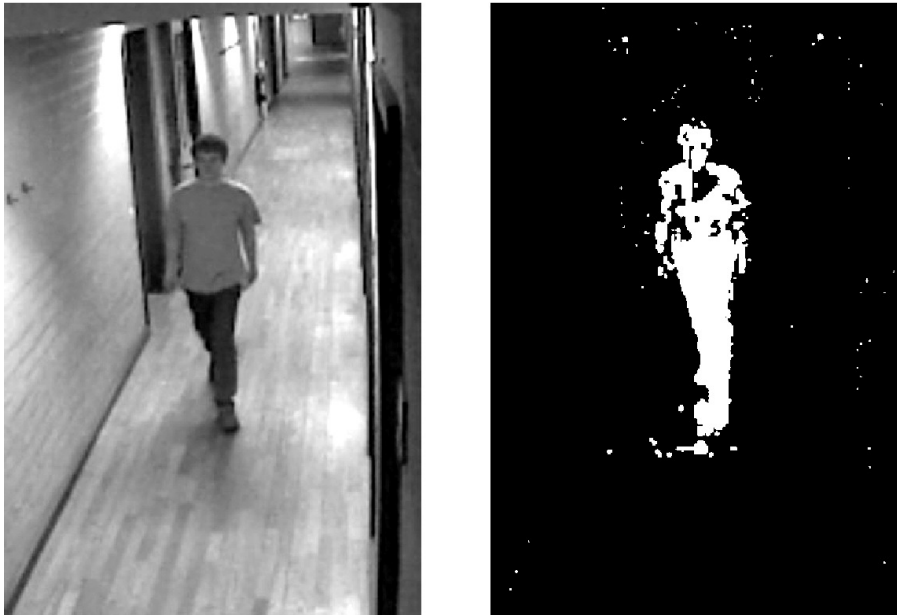
Figure 4.6: Example of binary silhouette extracted with the algorithm of Zivkovic, as described in [136].
