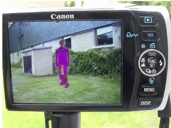
Figure 2.15: Embedded implementation of ViBe in a Canon camera.
