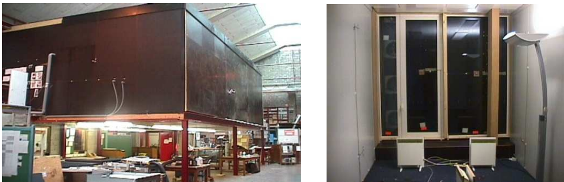
Figure 2.20: Climatic chamber: external and internal views
