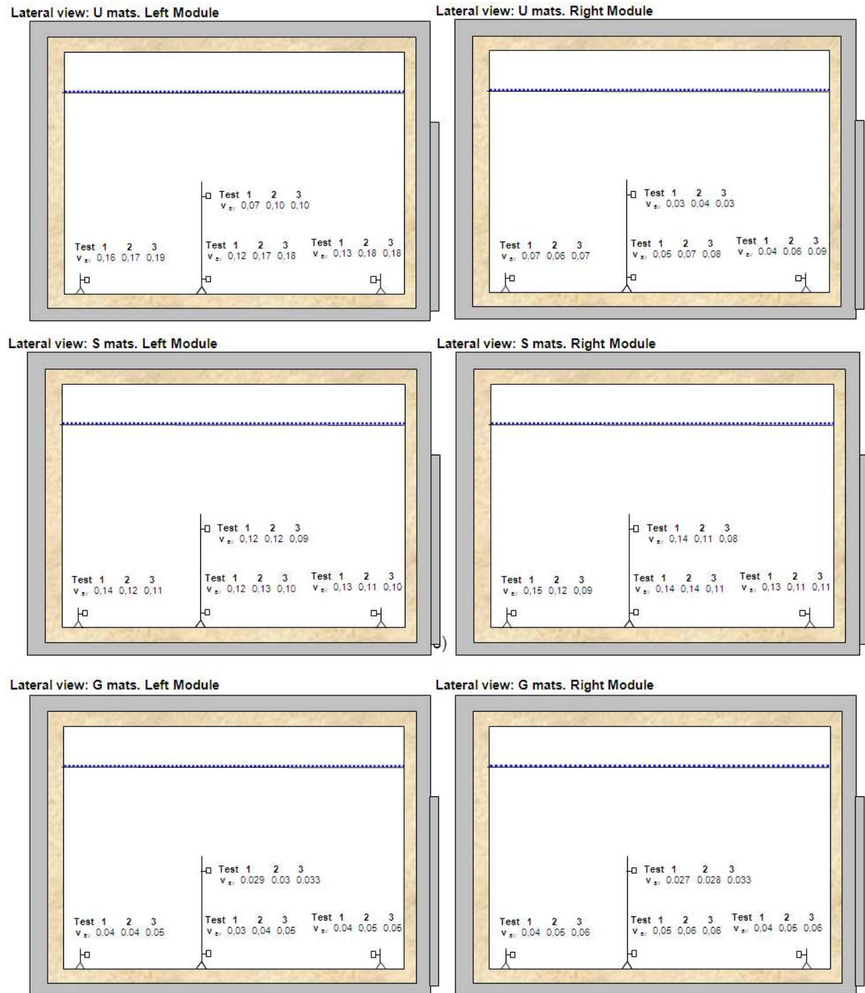
Figure 2.35: Air velocity measurement results for “U” “S” and “G” mats.
