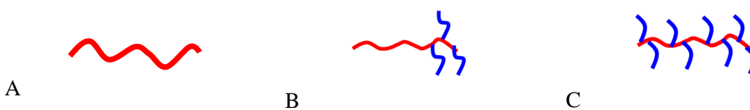
Fig. 3.1 Structure of homopolymers and copolymers employed in this study. The PDMAEMA backbone is represented in red and the PEG moieties are in blue. (A) PDMAEMA homopolymer (P1 and P2), (B) palm-tree PDMAEMA-co-MAPEG copolymer (P3 and P4), and (C) statistic-distributed PDMAEMA-co-MAPEG copolymer (P5).
