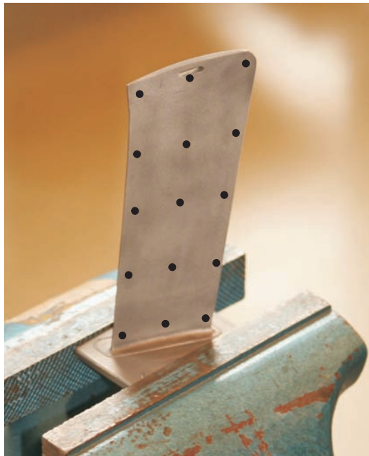
Figure 5.19: Experimental setup consisting of the stator blade caught in a vice. The bullets (●) refer to the measurement locations on the lower blade surface.
