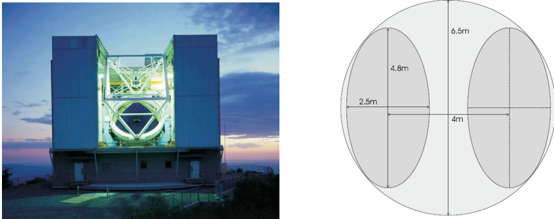
Figure 4.7: Left: Picture of the Multi-Mirror Telescope (MMT, Mount Hopkins, Arizona). Right: Division of the MMT pupil by the BLINC instrument to artificially produce a baseline of 4 m between two oval sub-pupils and perform destructive beam combination (Figure from Absil 2006).
