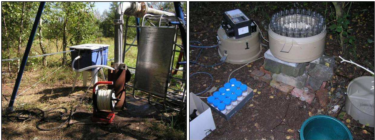
Figure 4.26. Radially converging flow tracer tests: experimental setup. Pumping device (left); automatic sampler (right).
