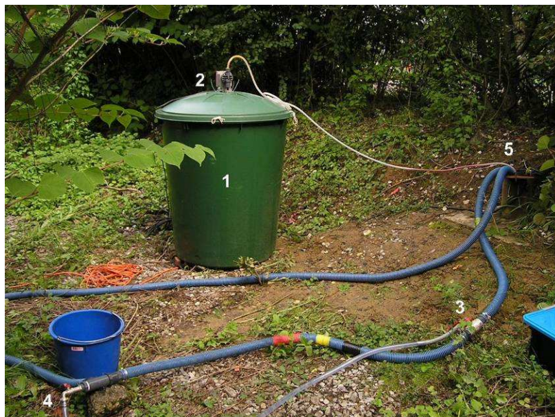
Figure 4.30. FVPDM: experimental design in the field during realisation of the experiment in well P3. (1) Tracer liquid tank; (2) Dosing pump; (3) Valve for control of the recirculation flow rate; (4) Tap for sampling operations; (5) Injection well (modified from Brouyère et al. , 2008).
