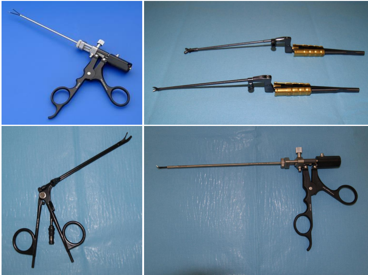
Fig. 3.3: Above left: example of single-shaft bipolar forceps with pistol grip designed for endoscopic surgery. Above right: example of coaxial scissors with rotatable blades and coaxial biopsy forceps. Bottom left: bipolar forceps allowing simultaneous aspiration at the upper tip of the forceps. Bottom right: same as above left but with curved tips, allowing for para-axial coagulation.
