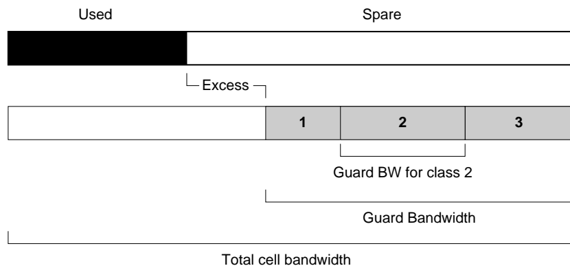
Figure 2.10: A call admission control procedure. Notice that there might be no “excess” bandwidth if the sum of the guard and the used bandwidth is greater than the cell capacity.
