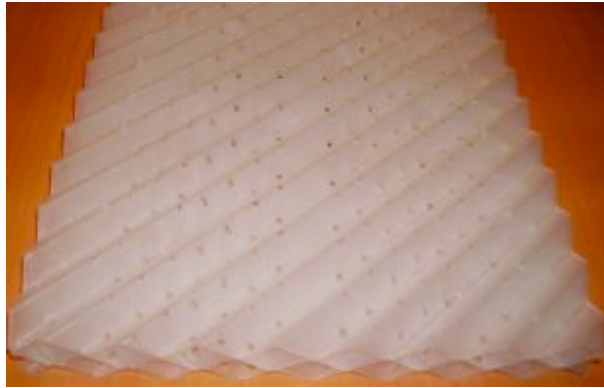
Figure 9.1: Example of structured packing used in distillation and reactive distillation columns.
