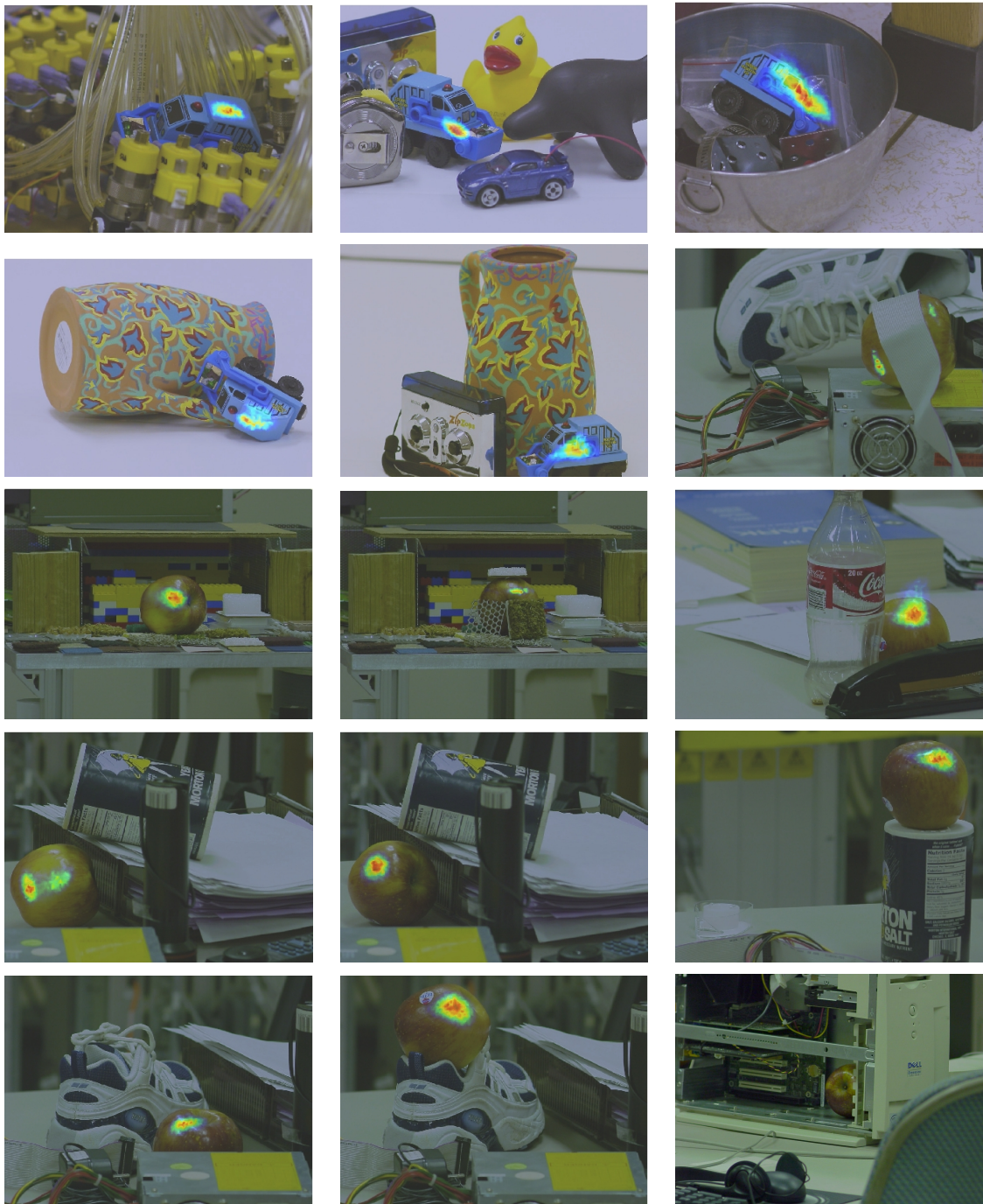
Figure 7.18: Examples of recognition of two objects in Ponce's object database [RLSP06]. The kernel density corresponding to the final belief (posterior marginals) after NBP are shown for the best features.
