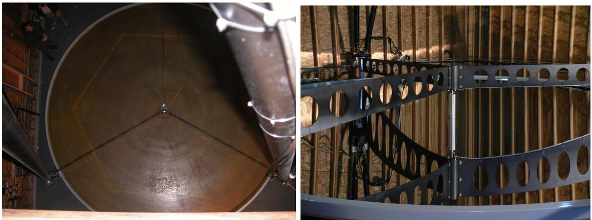
*Figure 1.24:* Left: The 6m mirror dish seen from the focal region. Right: Side view of the LZT 6m liquid mirror while it is rotating.
