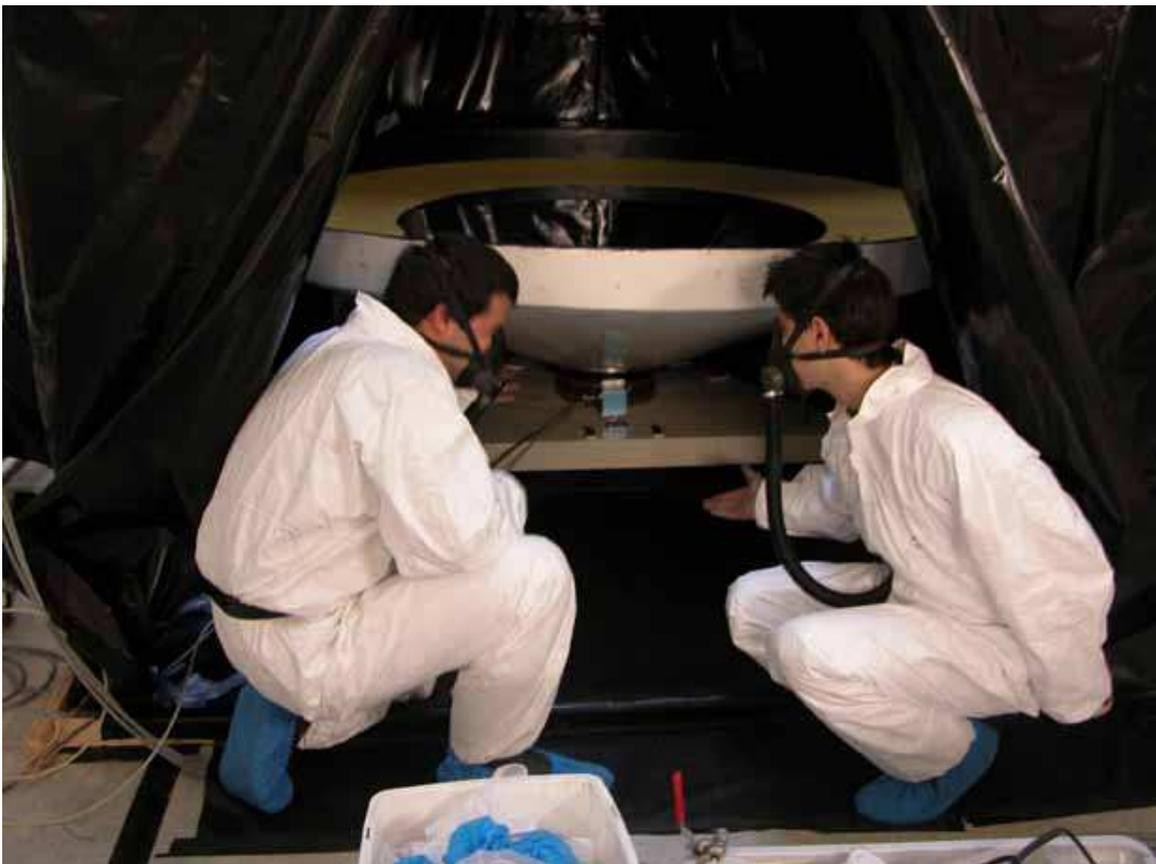
*Figure 1.10:* Mercury in the 2m LMT dish. A gas mask is necessary when working with mercury until an oxide layer has been formed on the surface. Gloves and protective suits are mandatory to avoid contamination. Davide Ricci and the author are seen on this photograph.
