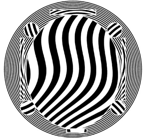
*Figure 5.11:* Example of multiplexed CGH. The central pattern creates the aspheric wavefront for surface testing. The outer regions are used to align the elements for the optical test (figure from Burge et al. 2007).
