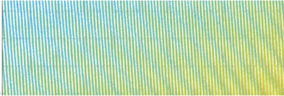
*Figure 2.15:* Image taken with the neon-ceiling lights of the room turned on. The vertical lines are interpreted as the signature of the 50Hz variation of the illuminating lights.
