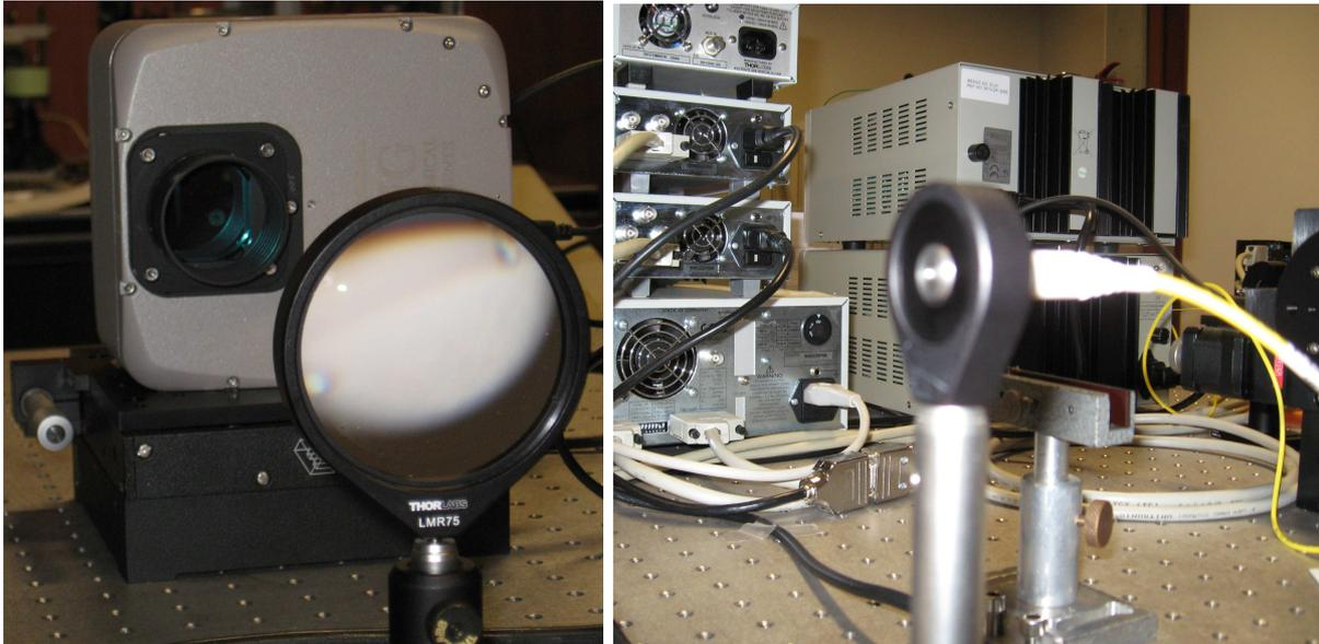
Figure 8.8: Left: the tested lens in front of the CCD camera. The latter is installed on a micro-control to fine tune its focal displacements. Right: the fiber source installed on its support. In the background, one can see the laser source itself with its cooling system and power supply.
