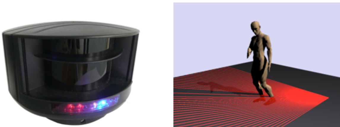
Figure 12: We use Range Laser Scanners (RLS, BEA LZR-i100, left) to produce a « curtain » horizontal and parallel to the ground, allowing the detection of feet position and their tracking as the subjects walks throughout the setting (right).
