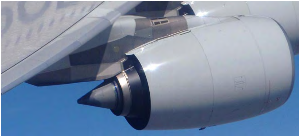
Figure 3.1: Pylon on the wing and the handed turbine engine (Airbus 380)
