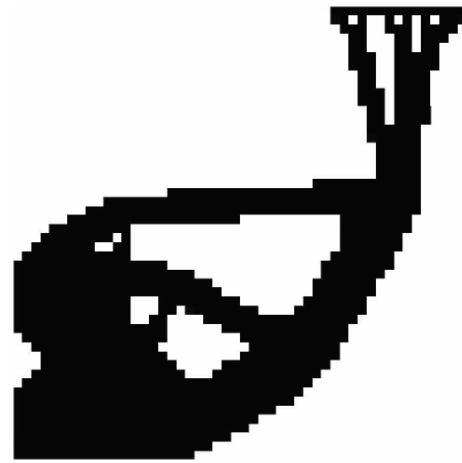
Figure 3.35: A regular topology optimization, 28.7kg, C = 0.0636J(2D)
