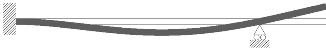
(a) 1 st natural frequency 17.15Hz
