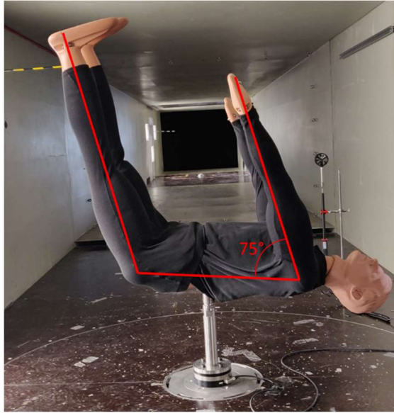
Figure 8: Mannequin in drownded position, tight clothing and yaw angle of 90°. Articulations blocked to have limbs with an angle of 75° with the horizontal.
