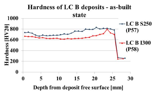
Figure 23 - Hardness of LC B S250 (P57) and LC B I300 (P58) deposits in as-built state. (Hashemi 2017).
