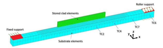
**Figure 4.** Initial symmetric mesh with the stored clad element (green) for future element activation, the mechanical boundary conditions in red (on the left, all the displacements x,y,z are fixed while on the right, only z displacements are prevented).
