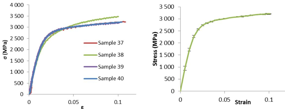
Figure 28 – a) True stress true strain curves of all the tested samples at room temperature and a strain rate of  $50 \times 10^{-3} \text{ s}^{-1}$ ; b) average cure with error bars from the samples 37, 39, and 40.
