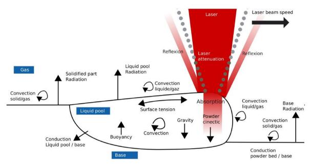
Figure 4 - Physical phenomenon during laser material interaction in DED (Marion 2016).
