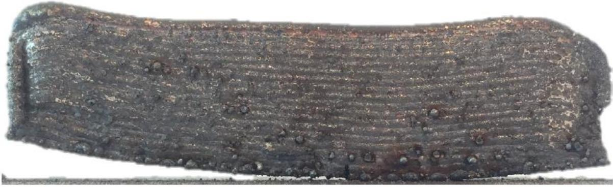
Figure 9 - Warpage of an DED part leading to its detachment from the substrate (Miedzinski 2017).
