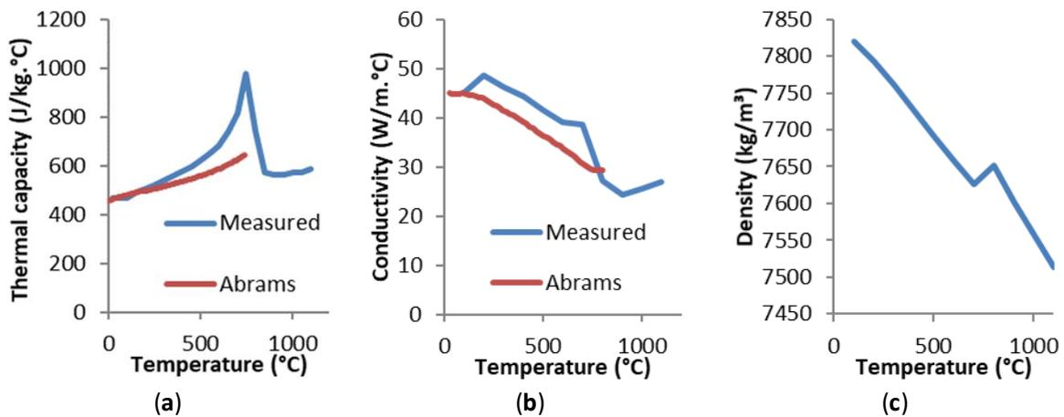
**Figure 8.** Thermo-physical properties of 42CrMo4: (a) thermal capacity,  $c_p$ ; (b) thermal conductivity,  $k$ ; (c) density,  $\rho$ . Measurements heating and cooling generating pearlite state at a rate of 3 °C/s.
