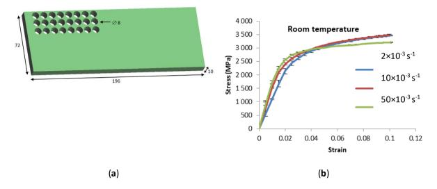
**Figure 11.** (a) Compression samples of Ø 8mm cut from a LMD-P sample of 196x72x10 mm; (b) True stress strain curves for different strain rates at room temperature.
