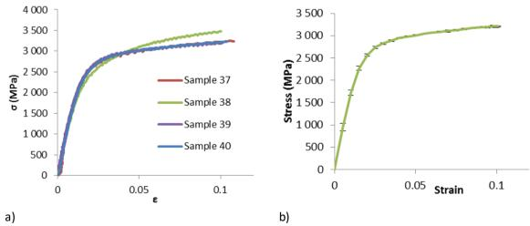
Figure 28 - a) True stress true strain curves of all the tested samples at room temperature and a strain rate of  $50 \times 10^{-3} \text{ s}^{-1}$ ; b) average cure with error bars from the samples 37, 39, and 40.
