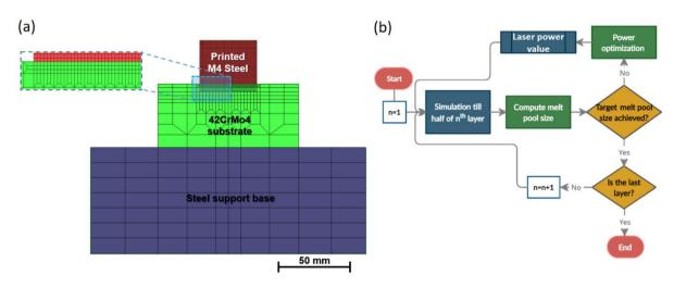
Fig. 5. (a) 2D FE Mesh used for DED process simulations and (b) flowchart of the laser power optimization process strategy for a constant melt pool size.
