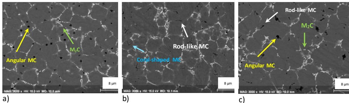
Fig. 3: SEM-BSE micrographs of a) POI1 with star-like MC and lamellar eutectic  $M_2C$  intercellular carbides; b) POI2 with coral-shaped intracellular MC, intercellular eutectic  $M_2C$ , and refined cells due to multiple melting; c) POI3 with coarse angular MC and eutectic  $M_2C$  within intercellular zones.
