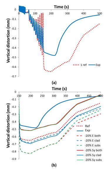
**Figure 18**. (a) Correlation between measured and predicted vertical displacements (- down, + up) during the cladding process, including the preheating and cooling stages. (b) Sensitivity analysis in the cooling stage to negative variations of Young's modulus (E) and the elastic limit (Sy) of the clad and the substrate.
