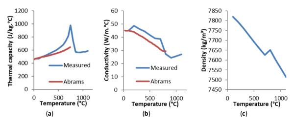
**Figure 8.** Thermo-physical properties of 42CrMo4: (a) thermal capacity,  $c_{\rho}$ ; (b) thermal conductivity, k; (c) density,  $\rho$ . Measurements heating and cooling generating pearlite state at a rate of 3 °C/s.
