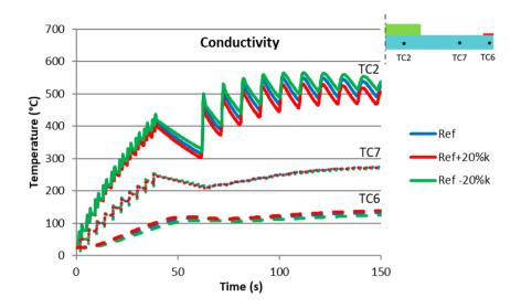
Figure 16. Sensitivity of substrate conductivity variation on the thermal history.
