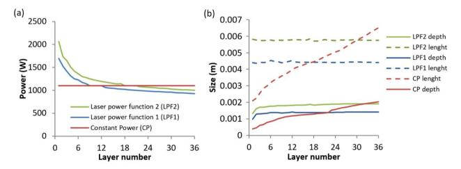
**Fig. 6.** (a) Laser power functions obtained from the proposed methodology. (b) Computed molten pool over the layers for LPF1, LPF2 and CP.
