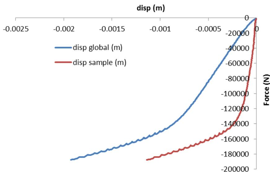
Figure 27 – Subtraction of the machine displacement over the global displacement at room temperature and  $50E-3 \text{ s}^{-1}$
