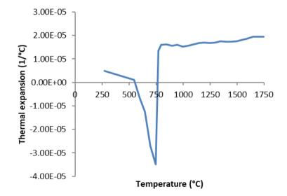
**Figure 9.** Thermal expansion coefficients for M4 from bulk sample (bainite/martensite) obtained with quenching cooling of 200 °C/s.
