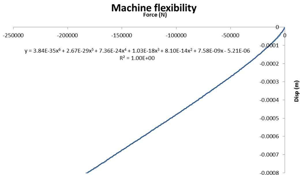
Figure 26 – Machine flexibility at room temperature for a strain rate of  $50E-3 \text{ s}^{-1}$
