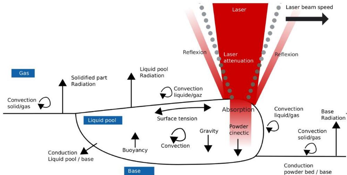
Figure 4 - Physical phenomenon during laser material interaction in DED (Marion 2016).
