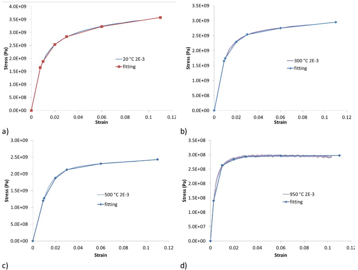
Figure 31 – Fitting of the stress strain curves at a) room temperature; b) 300 °C; c) 500 °C; d) 950 °C.
