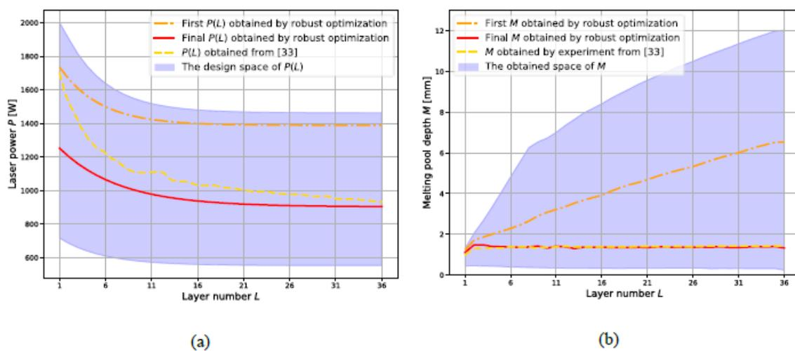
Figure 13 -  $P(L)$  and  $M$  are the laser power function and melt pool depth respectively used by T.Q.D. Pham in his DL approach in the M4 bulk sample studied in chapter 4 of the current thesis. a) comparison of  $P(L)$  identified by classical FE optimisation or DL for the same target of melt pool size, b) comparison of  $M$  evolution versus the different layers computed by both method associated to  $P(L)$  and verified by experiments.
