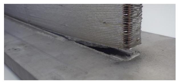
Figure 10 - Warping leading to build-part's detachment from the substrate/base-plate (Nain 2022).
