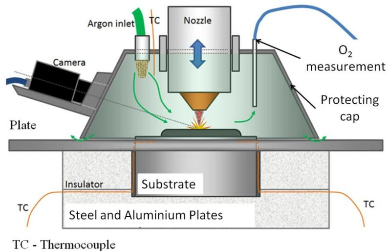
Figure 2 - Scheme of Sirris laser cladding equipment used for manufacturing thin wall and bulk specimens. (Hashemi 2017).
