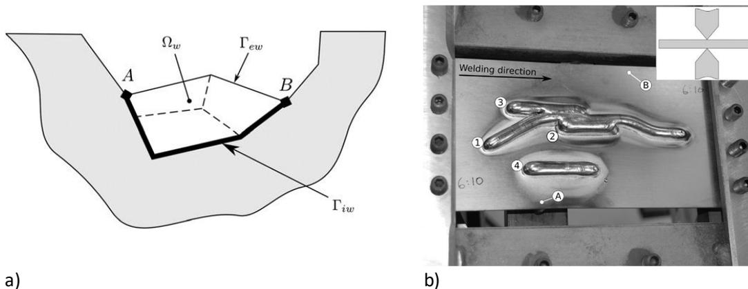
Figure 15 - a) Notation used for definition of weld geometry according to (Lindgren 2001); b) Validation part of (Saracibar 2014), complex thin wall of 10 layers.
