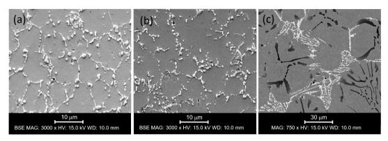
**Fig. 2.** SEM micrographs (BSE) show the ultrafine and cellular-type microstructures of DED AISI M4 sample manufactured with a constant laser power, (a) near the surface (within top layer), (b) at the sample mid height, and (c) BSE images of the coarse microstructure of a conventional cast sample (note the lower magnification of c image versus a and b ones).
