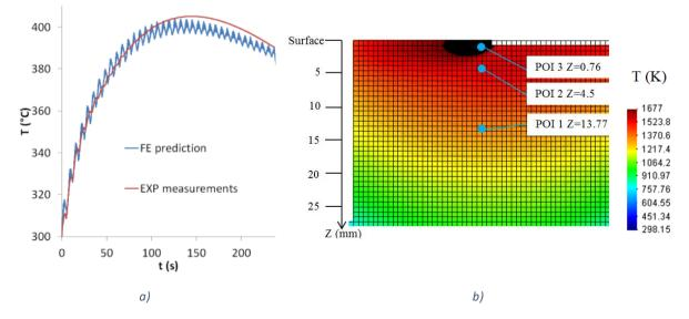
Fig. 1 a) Computed and experimental curves of temperature versus time at one thermocouple; b) FE thermal field during the last layer deposition (temperature higher than liquidus in black color) and location of points of interest (POI) within the thick deposit.
