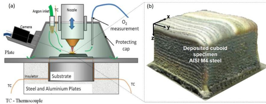
**Fig. 3.** (a) DED process used for the manufacturing of the bulk M4 samples, (b) Cuboid sample geometry and axes.
