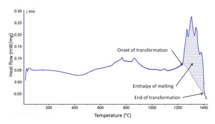
**Figure 7.** DSC measurement showing the latent heat of fusion of M4 (scanning rate of 3 °C/s).
