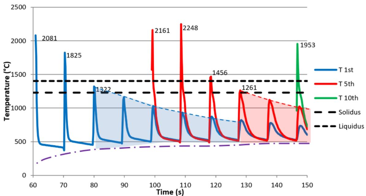
**Figure 14.** Thermal history of the 1<sup>st</sup>, 5<sup>th</sup>, and 10<sup>th</sup> deposits during the thin wall cladding process computed at a central point.
