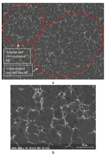
Figure 20 - SEM micrographs (BSE) showing the presence of coral-shaped and rod-like eutectic MC in the microstructure of LC B S250, a) 6.5 mm from the free surface, b) 4.5 mm from free surface (Hashemi 2017).
