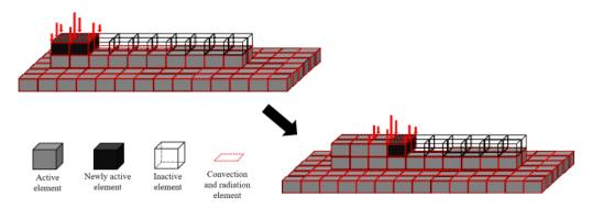
Figure 5. Schematic representation of the element birth technique.
