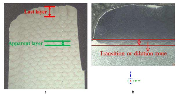
Figure 16 - a) deposit observed by binocular, b) deposit observed by optical microscope, showing the remelting effect of the substrate (transition or dilution zone) (Hashemi 2017).
