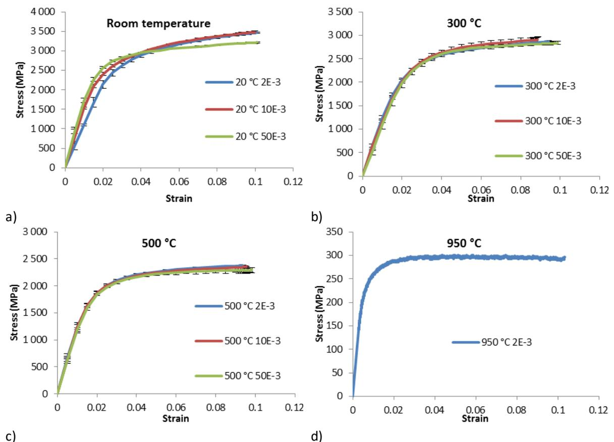
Figure 29 – Stress-strain curves at different temperatures and strain rates. a) room temperature; b) 300 °C; c) 500 °C; d) 950 °C.
