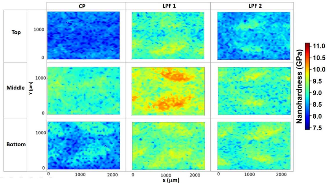
Fig. 9. Nanohardness maps of the cross-section of the samples at the top, bottom and middle location points.
