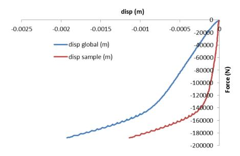
Figure 27 – Subtraction of the machine displacement over the global displacement at room temperature and 50E-3 s-1
