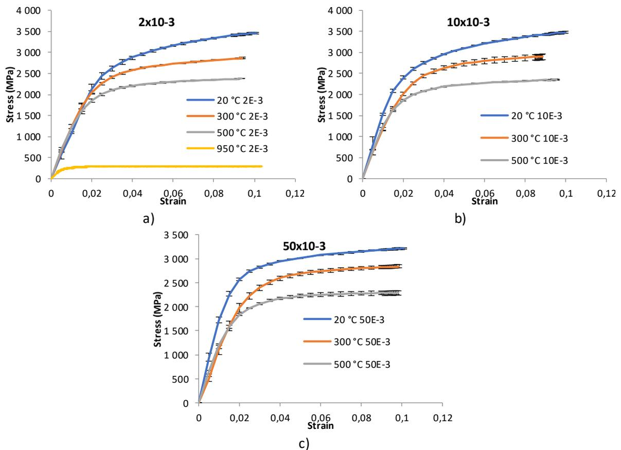
Figure 30- Stress-strain curves at different strain rates. a)  $2 \times 10^{-3}$ ; b)  $10 \times 10^{-3}$ ; c)  $50 \times 10^{-3}$ .
