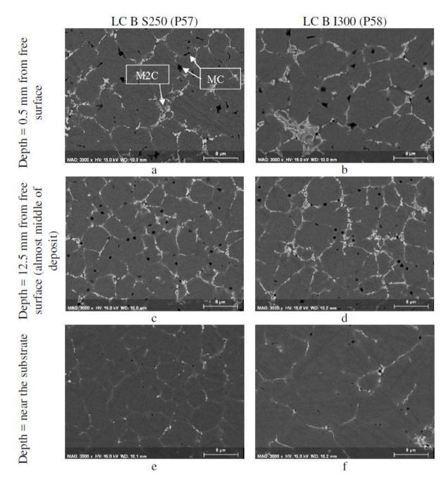
Figure 19 - SEM micrographs (BSE) showing the ultrafine microstructure of 2 LC B S250 (P57) and LC B I300 (P58) deposits, observed in 3 depths and in as-built state (Hashemi 2017).
