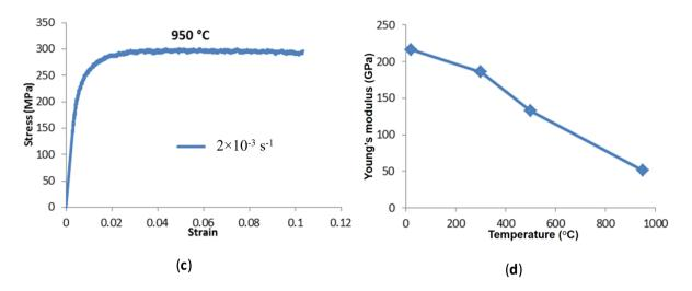
**Figure 12.** Stress strain curves at different temperatures and strain rates: (**a**) 300 °C; (**b**) 500 °C; (**c**) 950 °C; (**d**) Elastic modulus dependence on temperature for M4 DED material.
