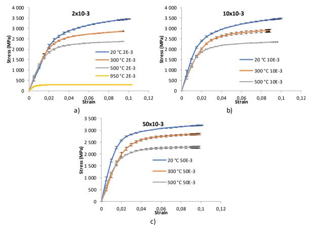
Figure 30- Stress-strain curves at different strain rates. a) 2x10<sup>-3</sup>; b) 10x10<sup>-3</sup>; c) 50x10<sup>-3</sup>.
