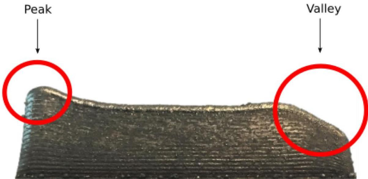
Figure 7 - Edge defects of a DED part (Miedzinski 2017).
