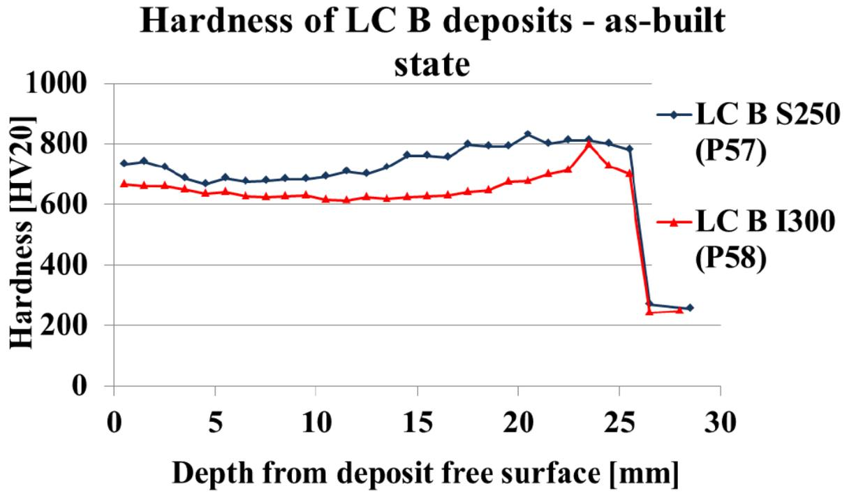
Figure 23 - Hardness of LC B S250 (P57) and LC B I300 (P58) deposits in as-built state. (Hashemi 2017).
