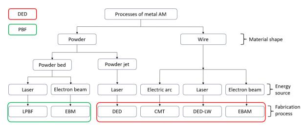
*Figure 1 – Different metal additive manufacturing processes (SLM now called LPBF), adapted from (Leroy-Dubief 2023).*
