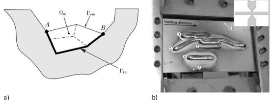
Figure 15 - a) Notation used for definition of weld geometry according to (Lindgren 2001); b) Validation part of (Saracibar 2014), complex thin wall of 10 layers.
