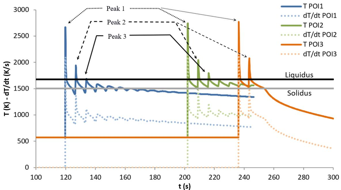
Fig. 2: Predicted curves showing the thermal histories (full lines) and temperature rate (dashed lines) within the three POIs.
