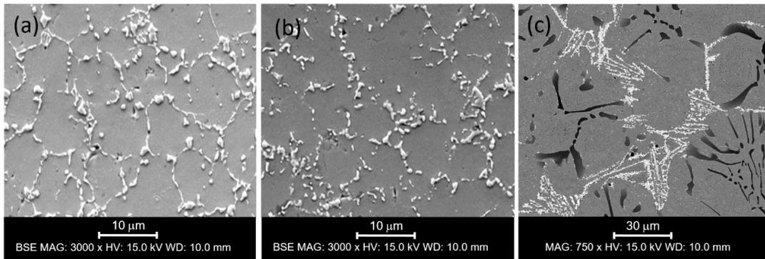
**Fig. 2.** SEM micrographs (BSE) show the ultrafine and cellular-type microstructures of DED AISI M4 sample manufactured with a constant laser power, (a) near the surface (within top layer), (b) at the sample mid height, and (c) BSE images of the coarse microstructure of a conventional cast sample (note the lower magnification of c image versus a and b ones).
