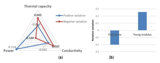
**Figure 19**. Summary of sensitivity analysis, expressed as the relative variation with respect to the reference case. (a) Thermal history sensitivity of the cladded sample with +-20% variations of thermal capacity, conductivity, and power. (b) Deflection sensitivity with -20% variation of Young's modulus and -20% of yield stress.
