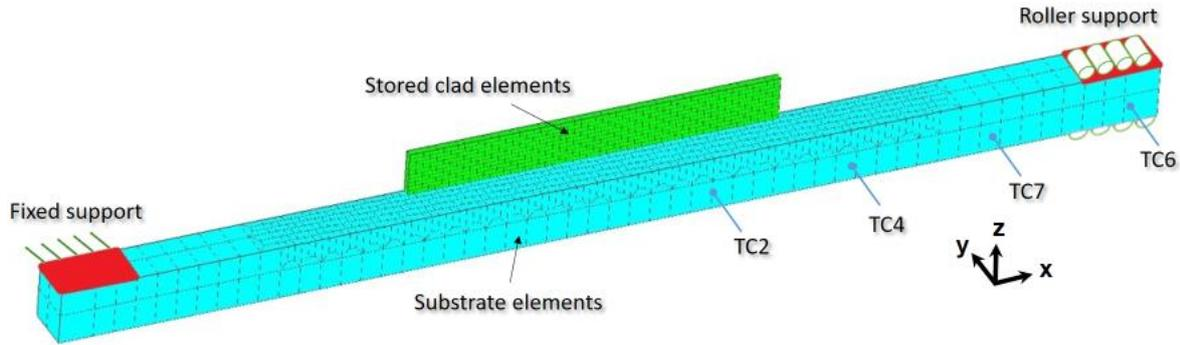
**Figure 4.** Initial symmetric mesh with the stored clad element (green) for future element activation, the mechanical boundary conditions in red (on the left, all the displacements  $x,y,z$  are fixed while on the right, only  $z$  displacements are prevented).
