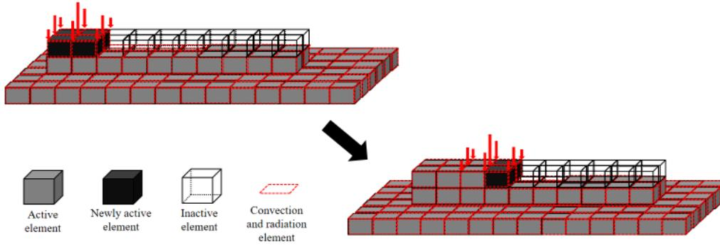
**Figure 5.** Schematic representation of the element birth technique.
