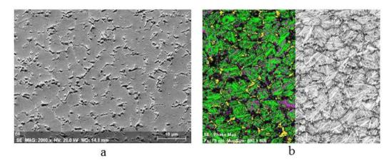
Figure 21 - a) Microstructure of LC B S300 deposit (sample P76), b) EBSD phase map of LC B S300 deposit in as-built state, showing distribution of Mo and W-rich M<sub>2</sub>C (yellow), V-rich MC (violet) and martensitic matrix (green) (Hashemi 2017).
