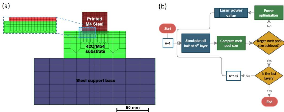
Fig. 5. (a) 2D FE Mesh used for DED process simulations and (b) flowchart of the laser power optimization process strategy for a constant melt pool size.
