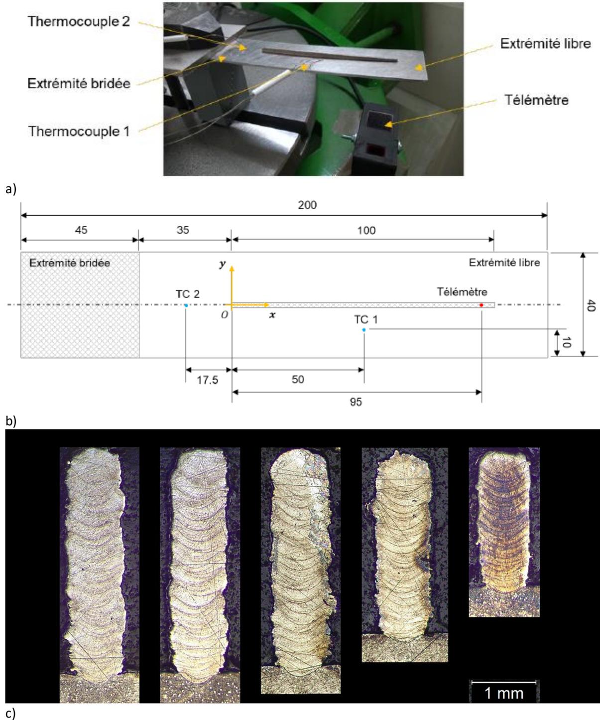
Figure 14 – a) Experiment design, b) Sample geometry and location of measurements, c) Cut in a thin wall in 316L of 20 layers manufactured by DED with the experimental design described in a- and b) (Dubief-Leroy 2023).
