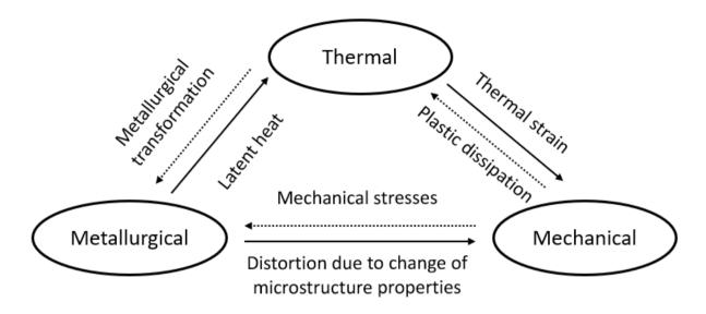
Figure 5 - Different physical phenomena happening in DED. Dotted line represents weak coupling and full line representing strong coupling. (Nain 2022).
