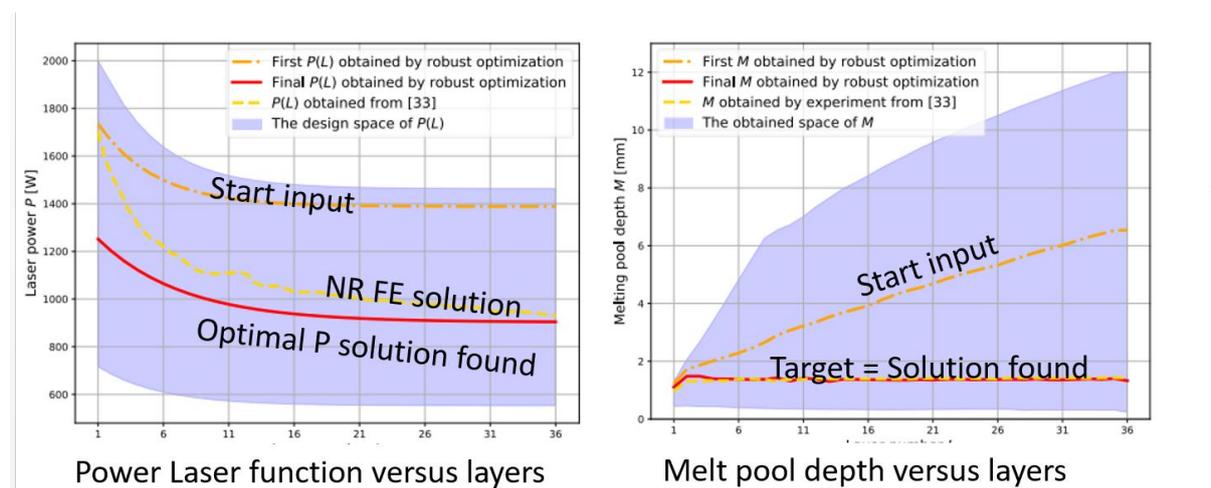
Figure 24 - Comparison of the laser power function  $LPF_2$  found by Newton Raphson (NR) in this research and the result of the robust optimization where the constant melt pool and an energy minimization define the objective function (Pham 2023). The start input information is associated with Pham's work.
