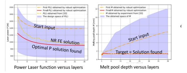
Figure 24 - Comparison of the laser power function LPF2 found by Newton Raphson (NR) in this research and the result of the robust optimization where the constant melt pool and an energy minimization define the objective function (Pham 2023). The start input information is associated with Pham's work.
