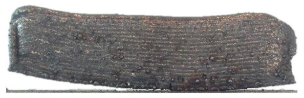
Figure 9 - Warpage of an DED part leading to its detachment from the substrate (Miedzinski 2017).
