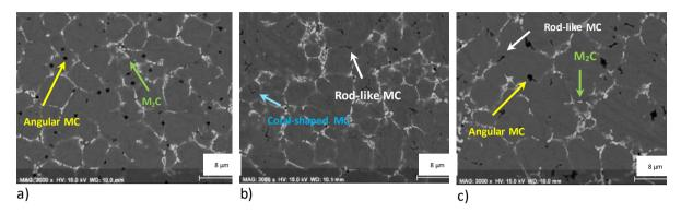
Fig. 3: SEM-BSE micrographs of a) POI1 with star-like MC and lamellar eutectic  $M_2C$  intercellular carbides; b) POI2 with coral-shaped intracellular MC, intercellular eutectic  $M_2C$ , and refined cells due to multiple melting; c) POI3 with coarse angular MC and eutectic  $M_2C$  within intercellular zones.
