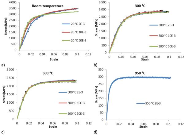
Figure 29 – Stress-strain curves at different temperatures and strain rates. a) room temperature; b) 300 °C; c) 500 °C; d) 950 °C.
