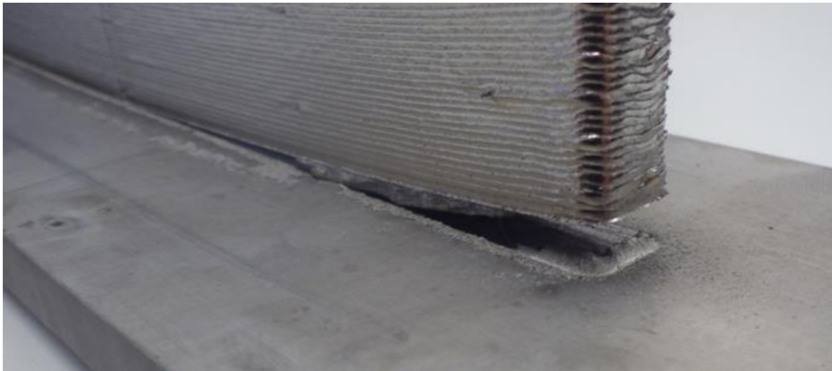
Figure 10 - Warping leading to build-part's detachment from the substrate/base-plate (Nain 2022)
