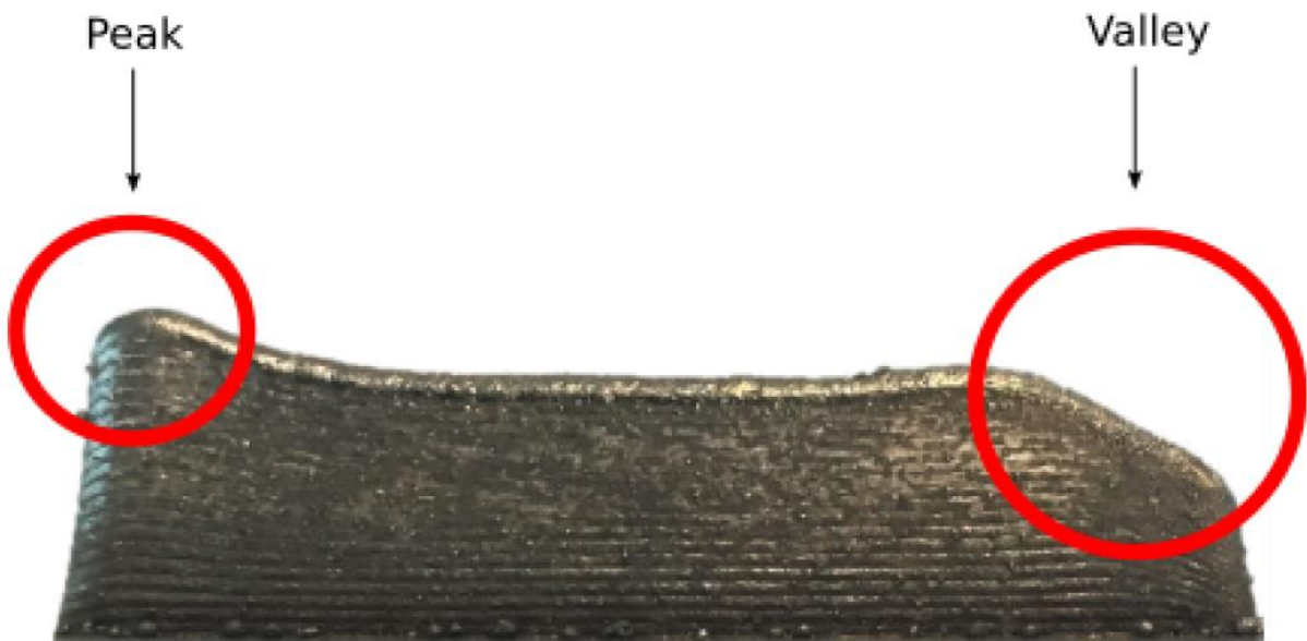
Figure 7 - Edge defects of a DED part (Miedzinski 2017).
