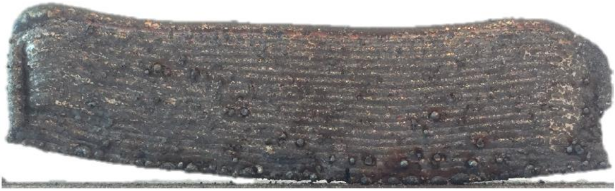
Figure 9 - Warpage of an DED part leading to its detachment from the substrate (Miedzinski 2017).
