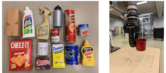
Fig. 5: (left) Object assets used in the real setup. (right) Successful grasp of a mug.
