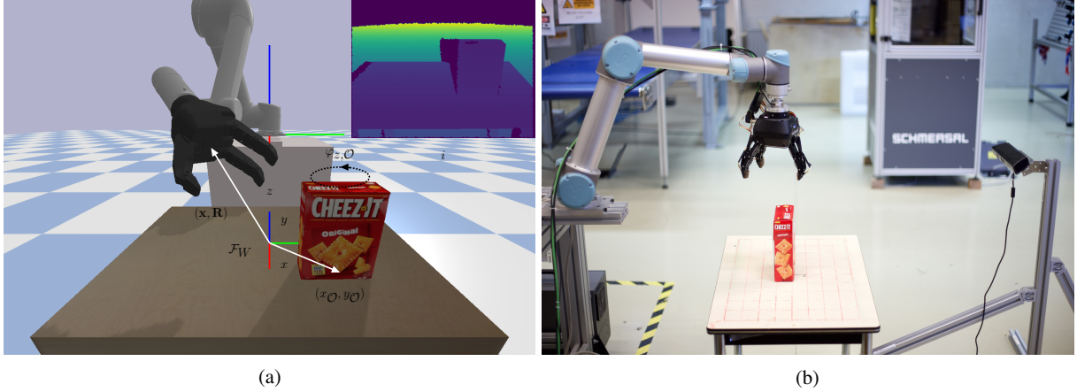
Figure 1: Our benchmark scene for multi-fingered grasping. The pose of the hand (\mathbf{x}, \mathbf{R}) is defined in the local object frame. The depth camera produces an image i of the scene.
