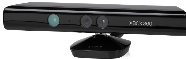
Figure 6.3: The Kinect. It produces 640 \times 480 depth images at the rate of 30 images per second.
