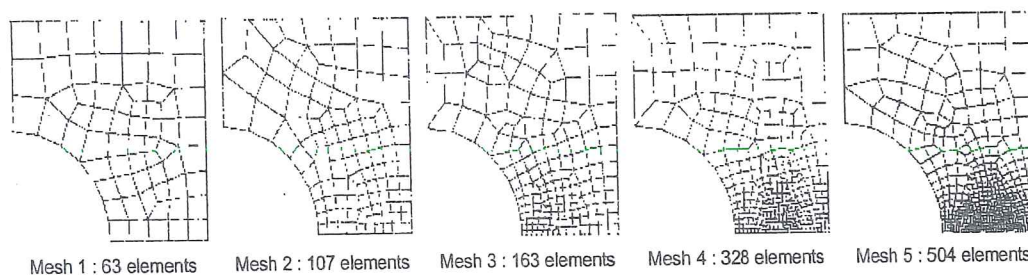
Figure 5-1 Meshes for the quarter plate (from de Vree et al. 1995).
