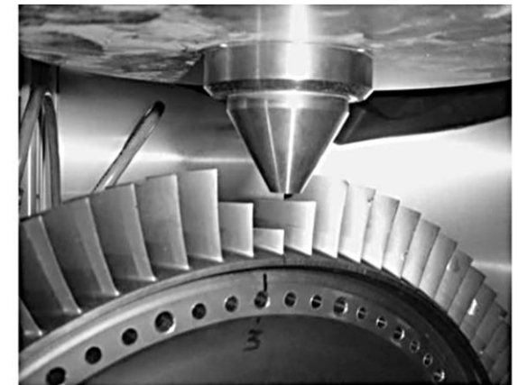
Titanium blisk repairing 4 Nowotny J. Therm. Spray Technol. , 2007
