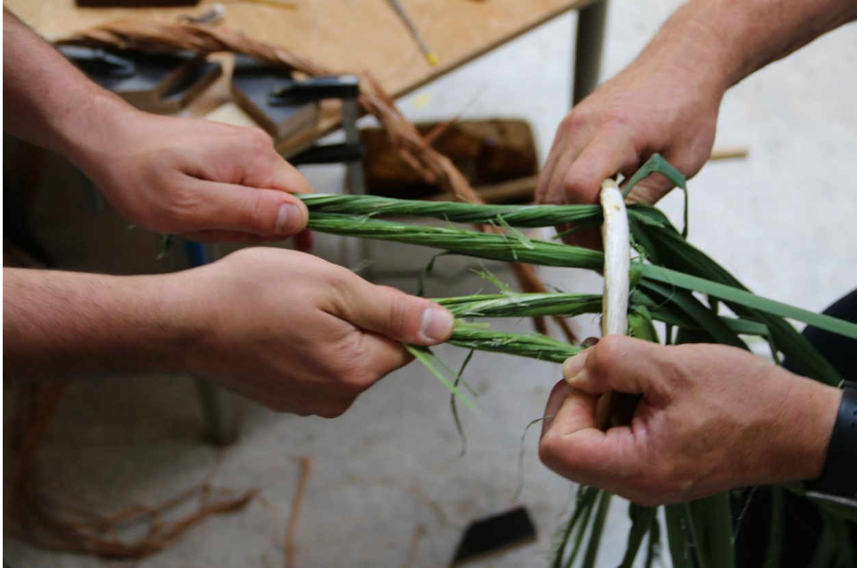
Fig. S14. Pulling the Typha through the holes and rotating fibres into strands by hand.
