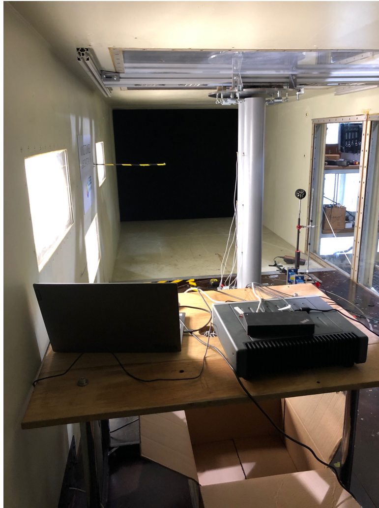
FIGURE 6.4: Picture of the experimental set-up to perform the modal analysis of the structure.
