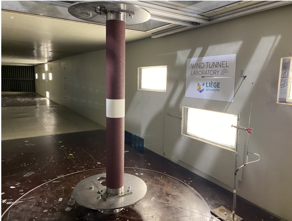
FIGURE 3.3: Picture of the experimental model of a single cylinder in the wind tunnel of Uliège.
