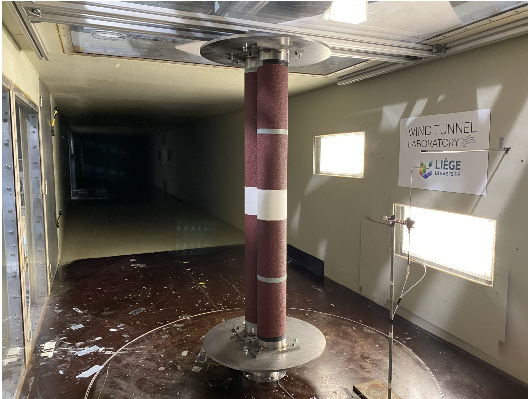
FIGURE 4.2: Picture of the experimental model of twin cylinders in the wind tunnel of Uliège.
