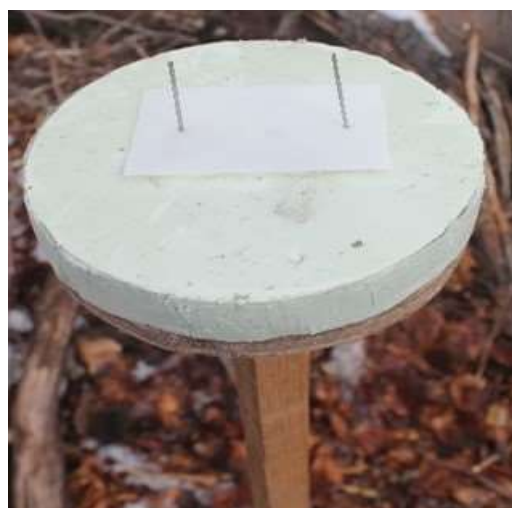
Figure 2. Passive spore traps used for the collection of spores of Fomes inzengae in beech stands.
