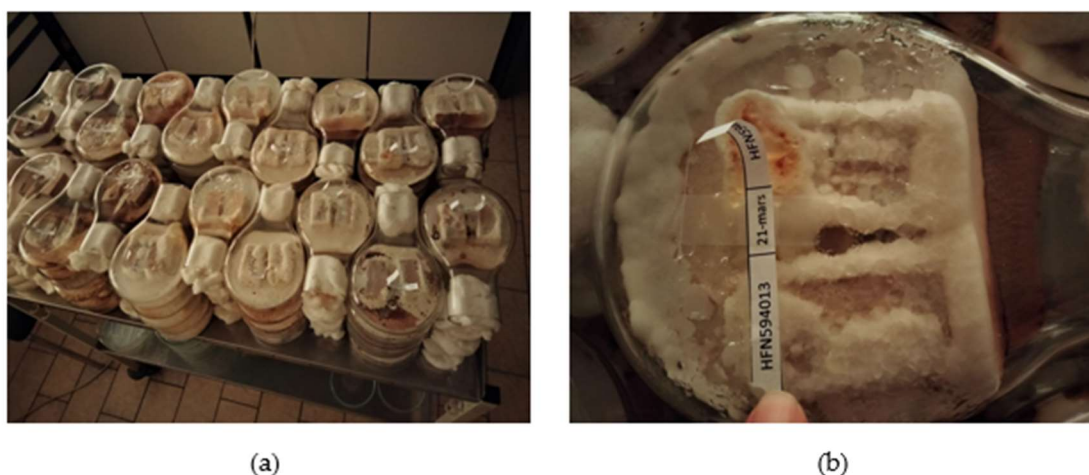
Figure 5. (a) Experiment in Kolle flasks to evaluate the wood decaying capacity of two isolates of F. fomentarius s.s. and two isolates of F. inzegae ; (b) wood specimen covered with mycelium after 16 weeks of incubation.
