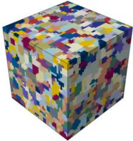
Representative Volume Element (RVE) synthetic microstructure.
