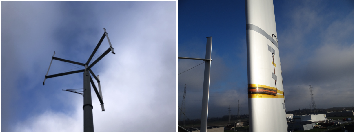
Figure 2. Pictures of the VAWT (left) and the WAMB device installed on one of its blades (right).
