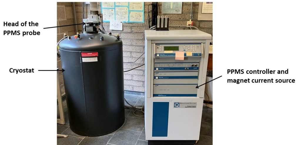
Figure 3.14: Picture of the Physical Property Measurement System (PPMS) including the cryostat and the control unit.
