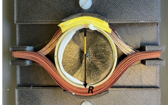
Figure 6.4: Picture of the hybrid screen. Two half bulk GdBCO cylinders are surrounded by a stack of 2G CC tapes in closed loop with an opening radius R = 17.5 mm.
