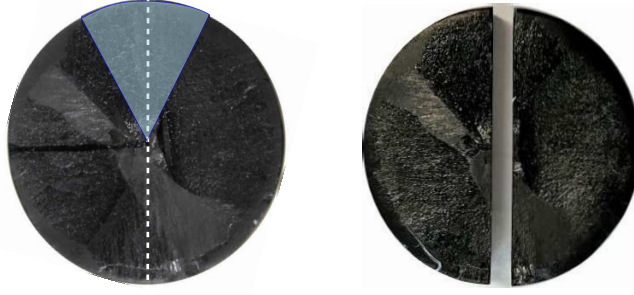
Figure 6.5: Pictures of the plain C001 GdBCO bulk cylinder (left) and the bulk cylinder after cut. The blue zone on the left picture shows the possible location of the macroscopic defect described in Section 4.1.2. The white dashed line shows the cut direction.
