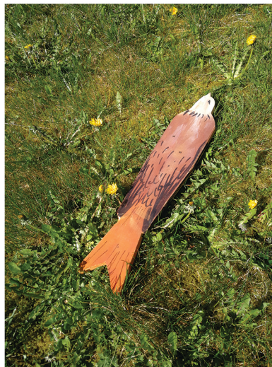
Red kite lure for searcher efficiency tests
