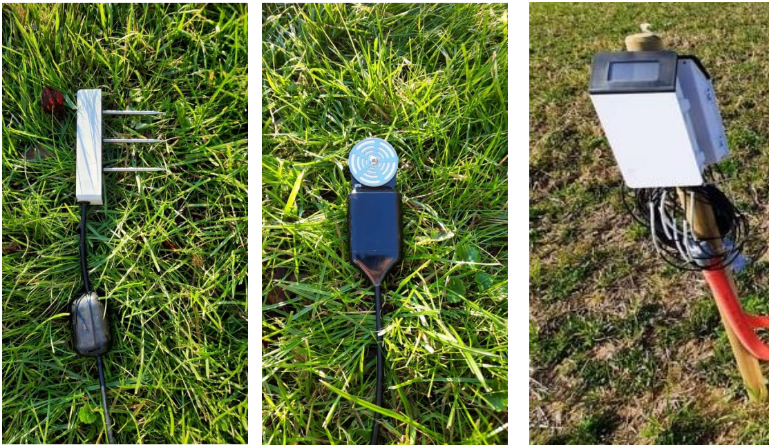
Figure 2. Sondes Teros 12, 21 et data logger ZL6
