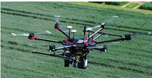
Figure 2. The DJI Matrice 600 with the YellowScan Surveyor LiDAR mounted below it.
