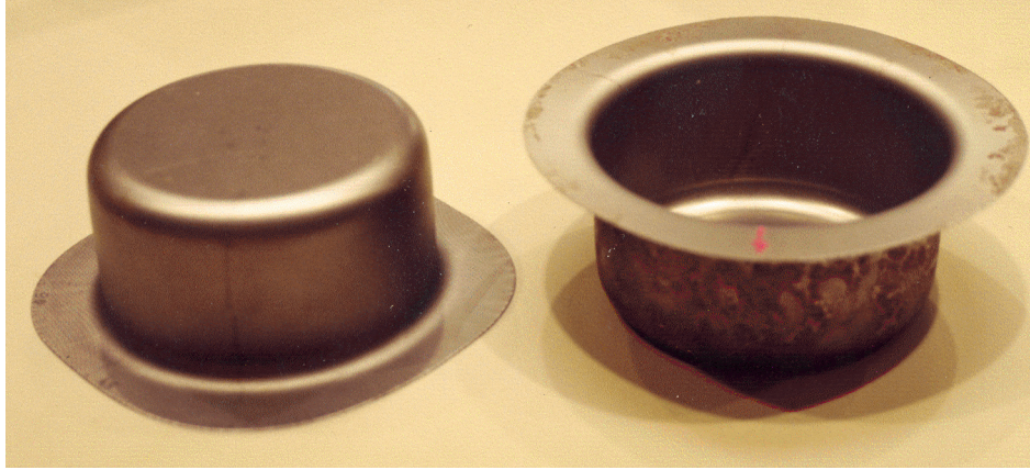
Figure 2.2: Cups produced by the deep drawing process; picture courtesy of Laurent DUCHÊNE (ULg)
