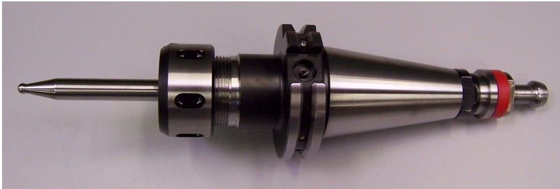
Figure 3.9: 5-mm tool inserted in the tool holding fixture; picture courtesy of Johan VERBERT (KUL)
