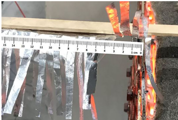
Figure 19. The zone of convective influence coming from the heating pads—qualitative measurement using a flag made of aluminium thin foil.
