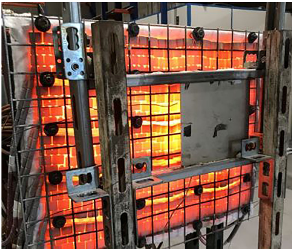
Figure 12. Test on stainless steel specimen: temperature difference visible on the surface of the heating pads through difference in the colour of the ceramic elements.
