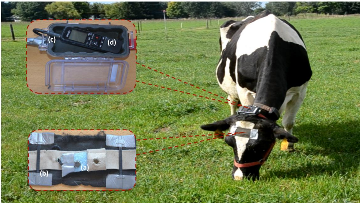
Figure 1. Recording system used to record the acoustic signals composed of inward and outward facing microphones (a). Wired microphones were covered by an elastic headband (b) and plugged (c) to a recorder housed inside a weather proof case attached to the top side of a halter neck strap (d).
