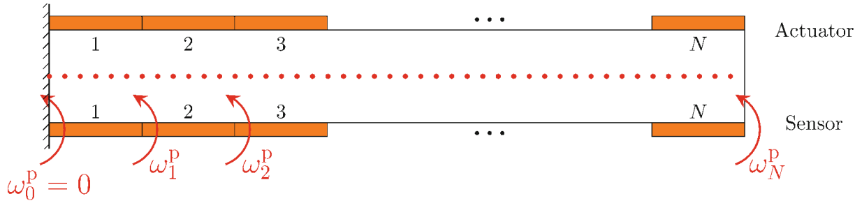
Figure 11.4 Beam covered with N pairs of collocated piezoelectric patches
