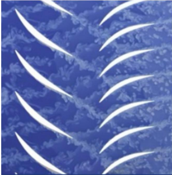
Scale resolving simulations DNS, LES and Wall modeled LES Months on O(10k) - (100k) processors No or little modeling
