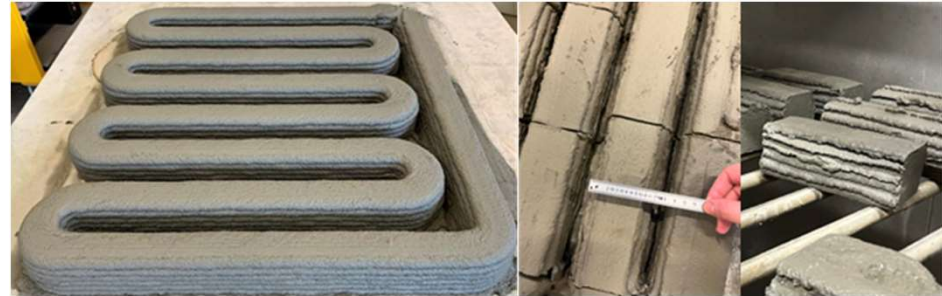
Printed samples (4x4x16 cm prismatic samples are extracted from S shaped printed éléments)
