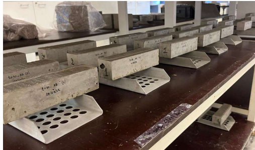
Casted samples (4x4x16 cm prismatic samples are casted)
